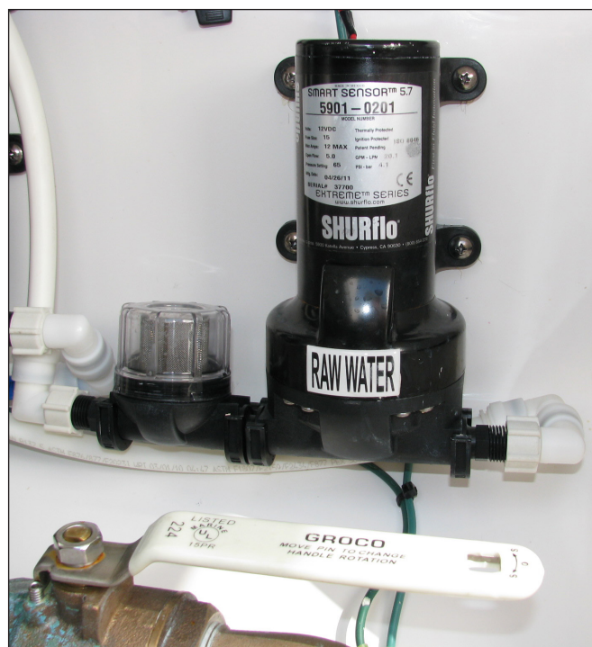
325 Center Console Fresh Water Pump and Strainer
