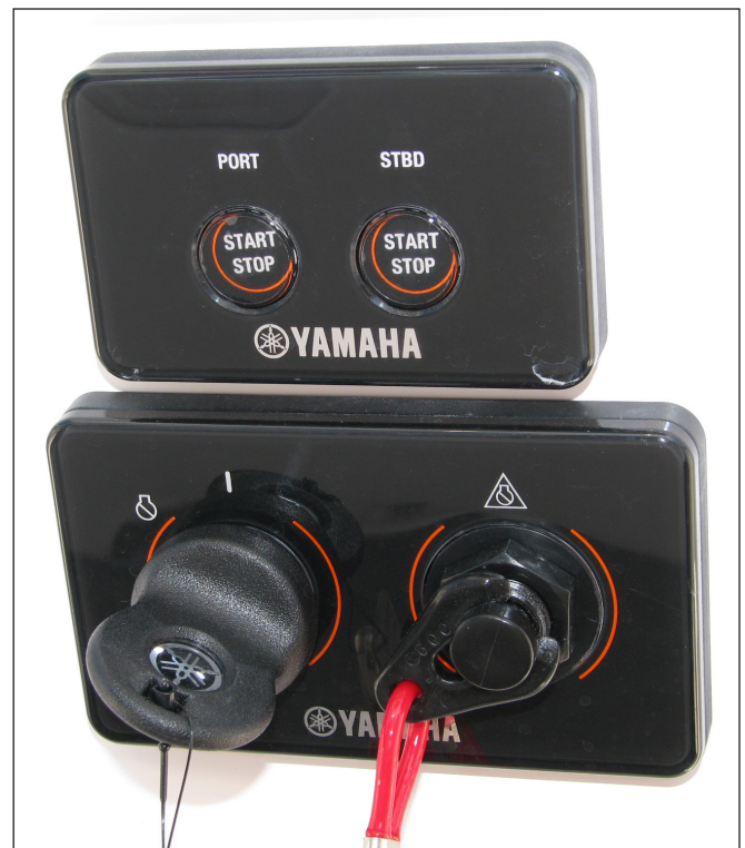
Typical Yamaha Command Link Ignition and Engine Start/Stop Switch System
