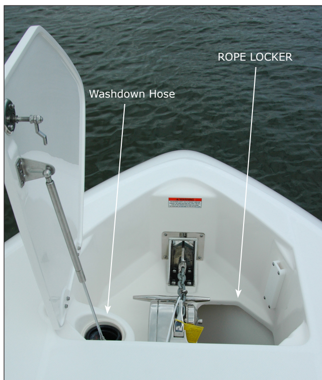
325 Center Console Anchor/Windlass Compartment
