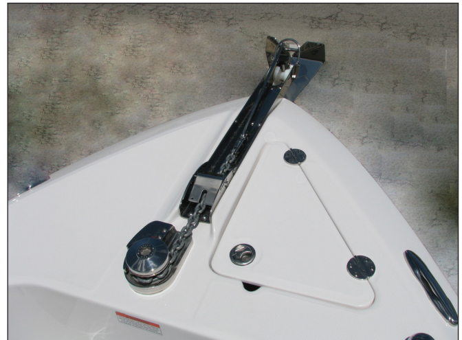
255/275/295 Center Console Anchor Roller Assembly, Windlass and Rope Locker
