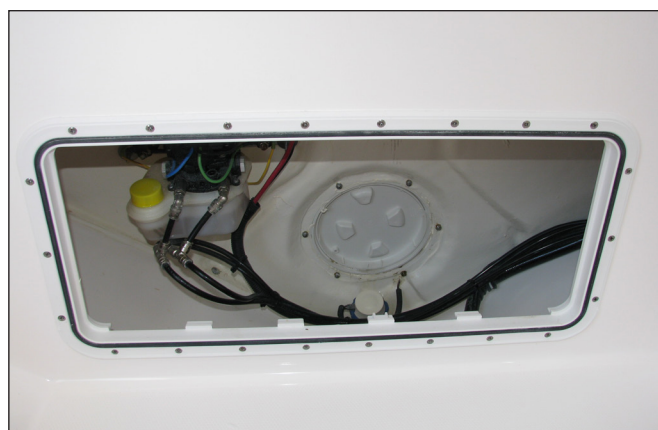
275 Center Console Forward Access Hatch, Windshield Hydraulic System and Fishbox Pump Out
