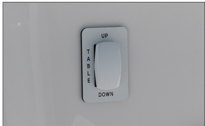
325 Center Console Table Pedestal Control Switch
