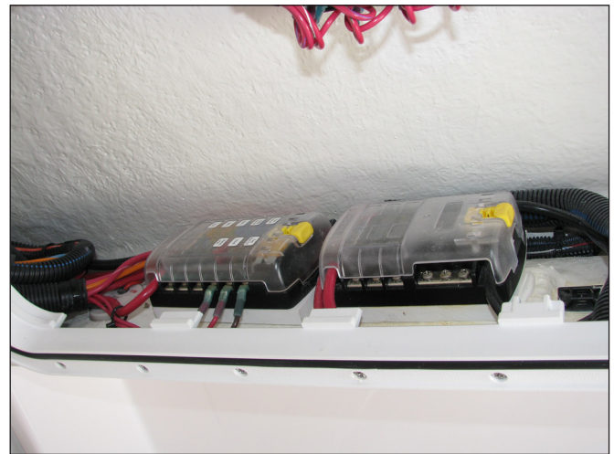
Typical Electronics and Helm Fuse Panels 255/275/295 Models
