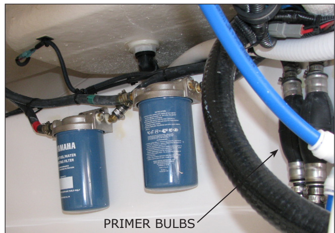
325 Center Console Fuel Filters and Primer Bulbs
