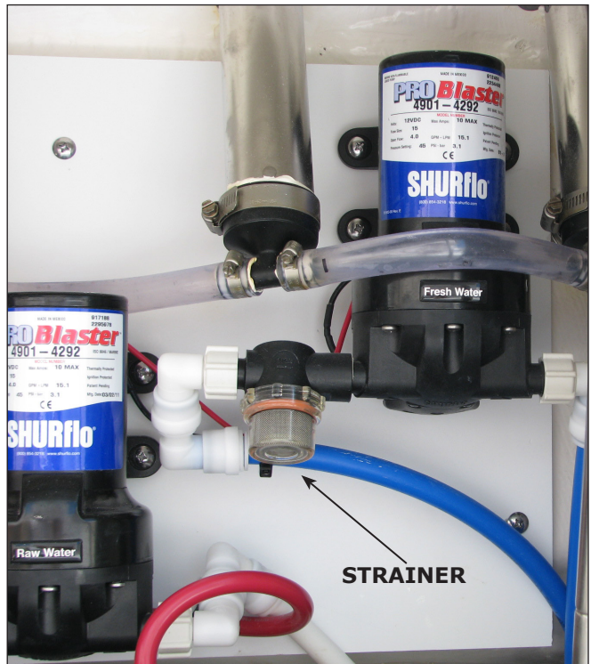
275/295 Center Console Fresh Water Pump and Strainer
