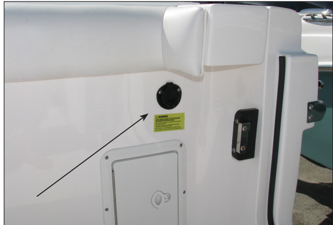
325 Center Console Shore Power Inlet Connection
