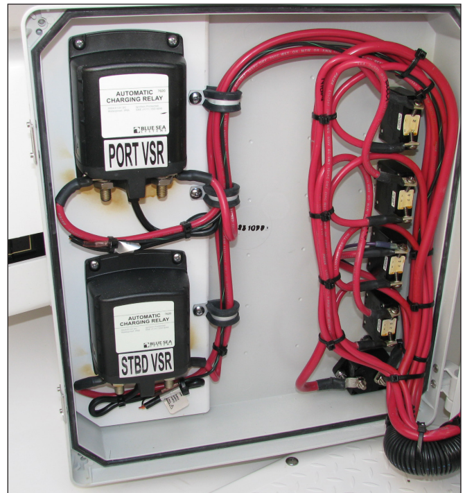
325 Center Console Voltage Sensitive Relays
