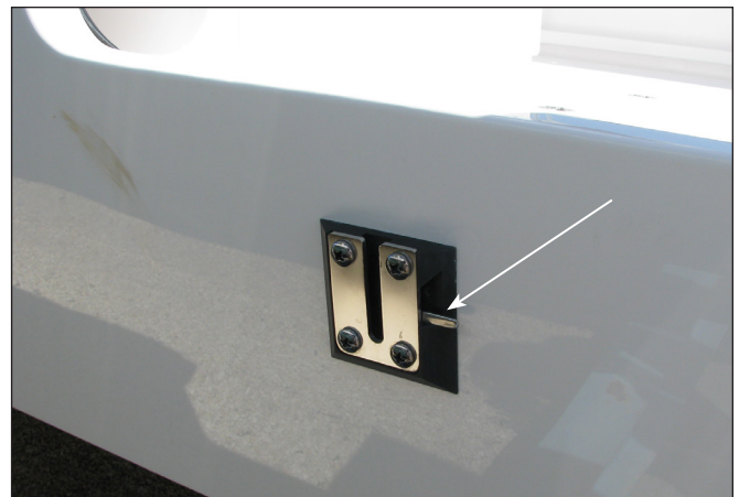
Dive Ladder Bracket and Release Lever
