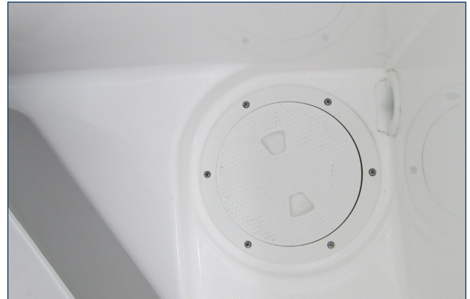
Forward Bilge Access Hatch
