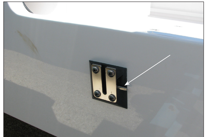
Dive Ladder Bracket and Release Lever
