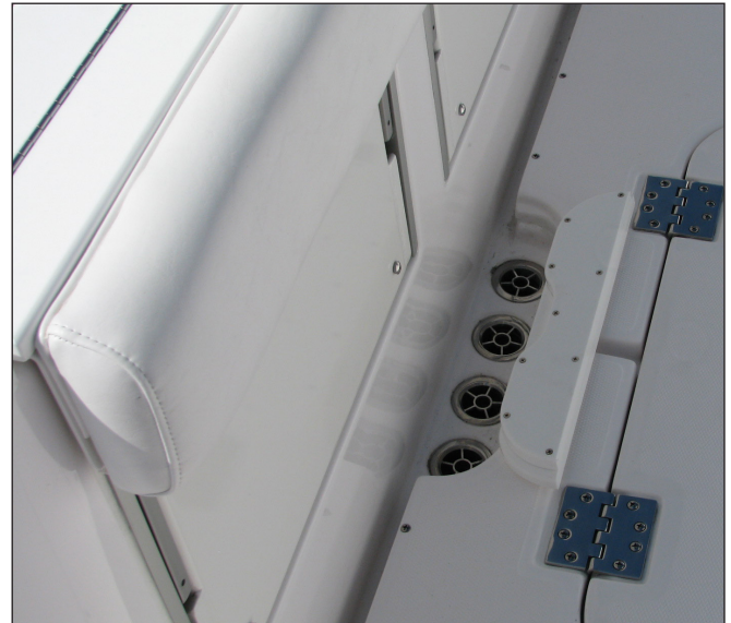
Typical Scupper Drains and Drain Rail
