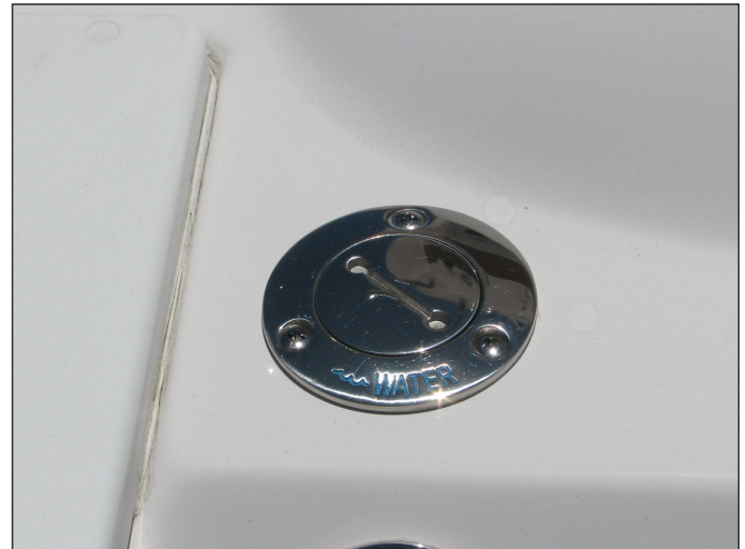
Fresh Water Fill
