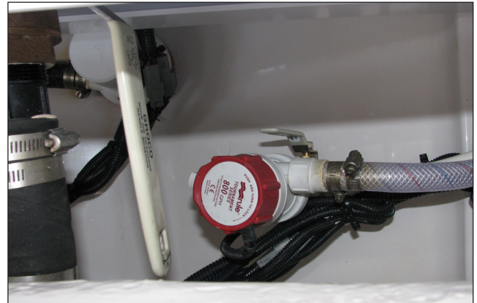
255/275/295 Center Console Baitwell Supply Pump and Seacock
