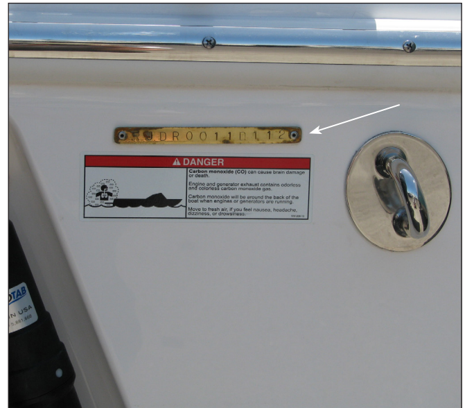
Hull ID # On Starboard Side of Transom
