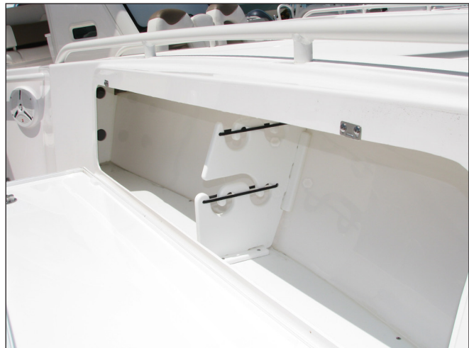
Typical Rod Locker at Bow
