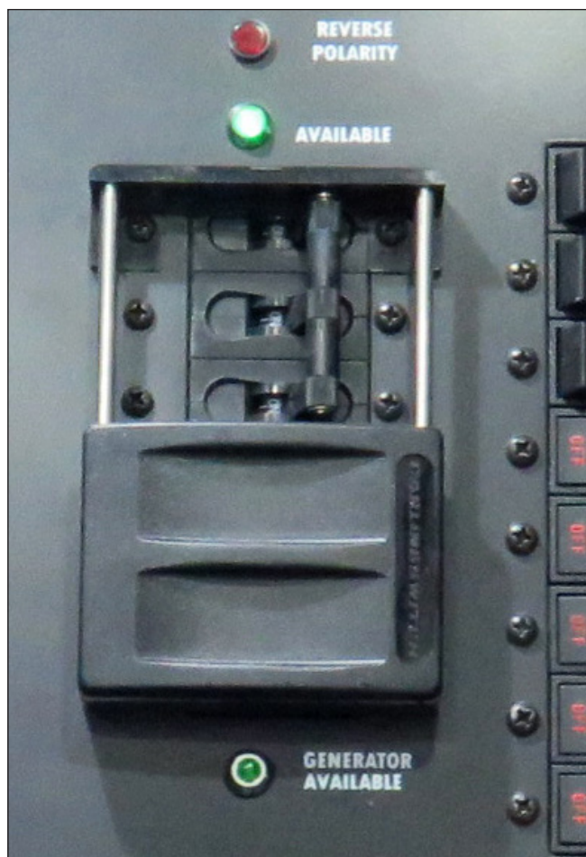
Reversed Polarity Light, Power Available Lights & Shore Power/Generator Main Breakers
