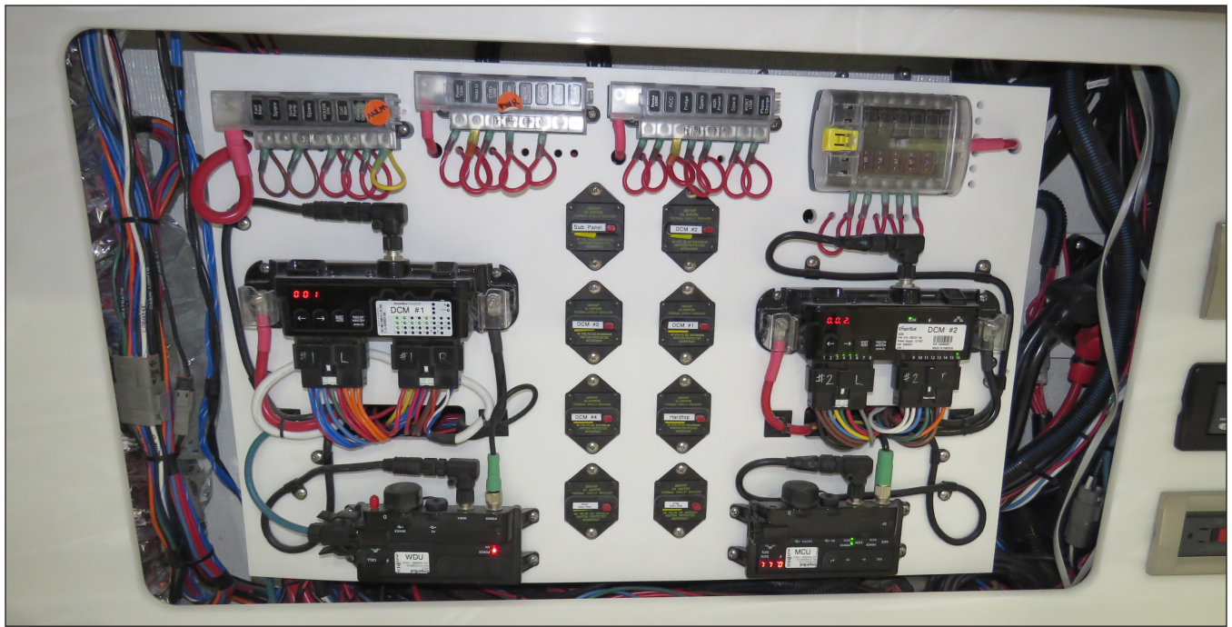
Digital Switch Control Modules & Main Circuit Breakers
