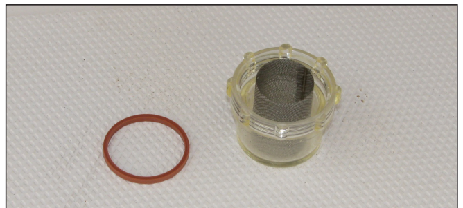
Typical Raw Water Pump Strainer Removed for Cleaning
