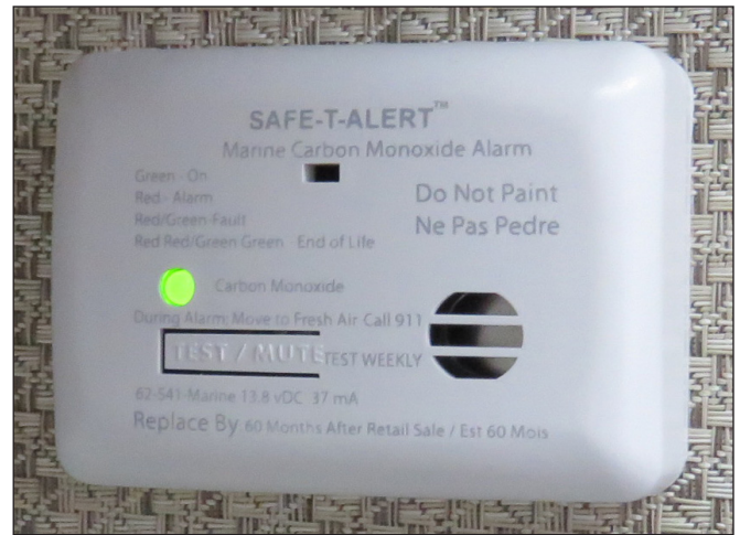
Typical Cabin Carbon Monoxide Detector
