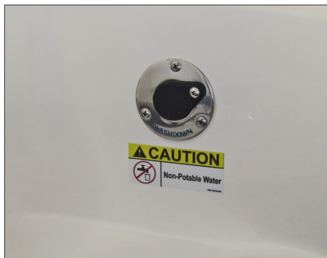
Typical Fresh Water Washdown Quick Connection
