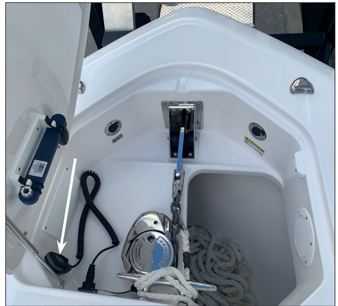
Windlass Control Switch
