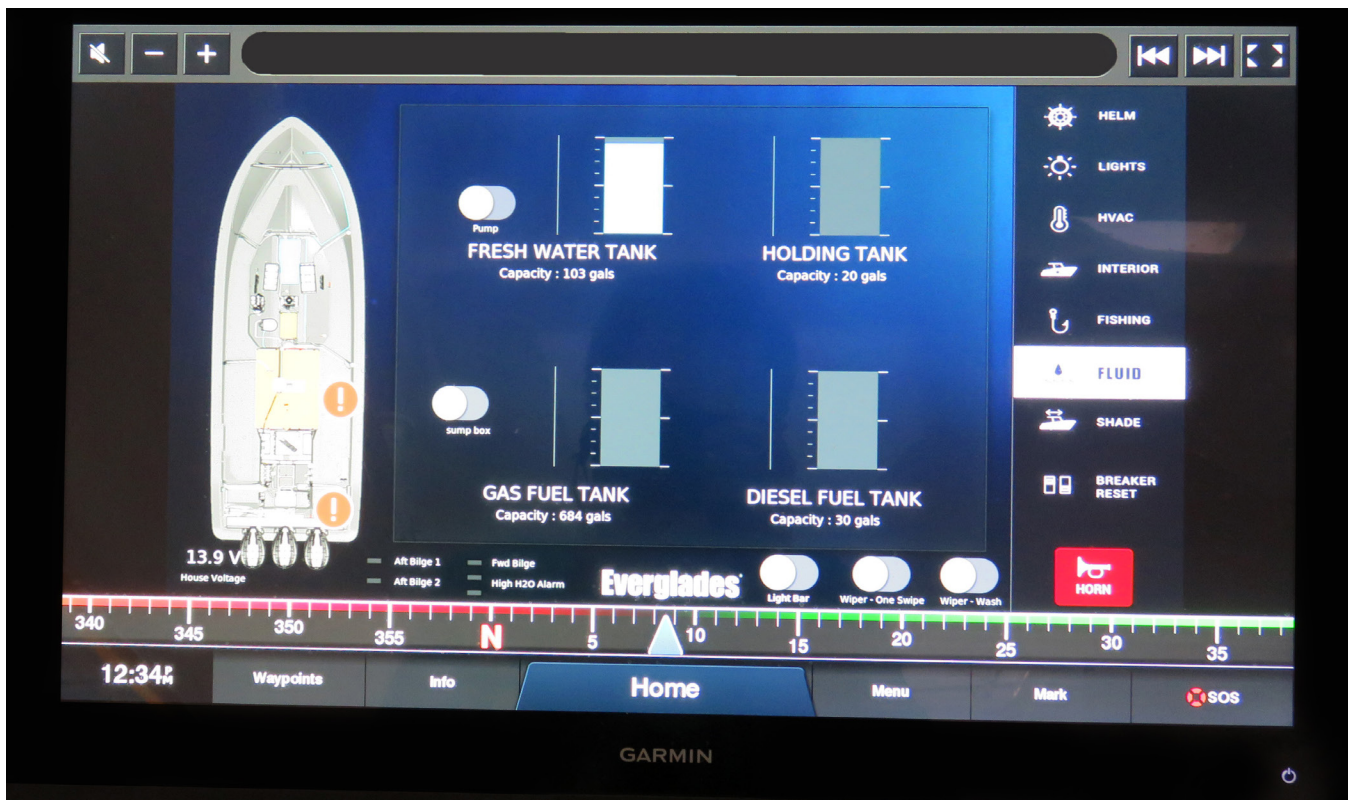
Fluid Level Monitoring Screen
