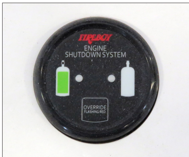
Fire Extinguisher Panel In Helm
