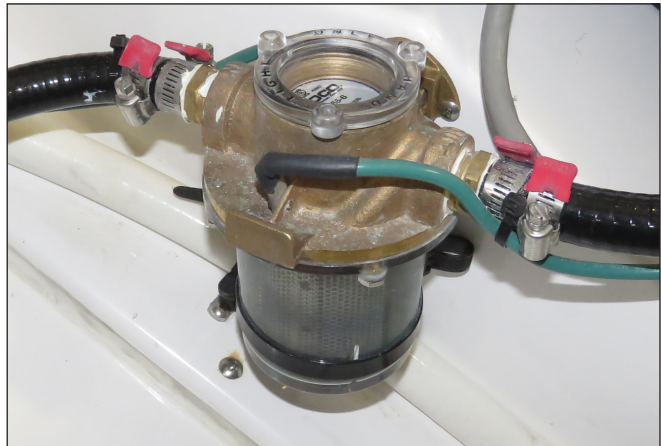
SeaKeeper Pump Sea Strainer
