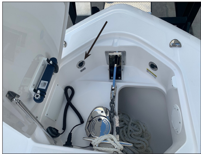
Windlass Raw Water Washdown Hose Connection
