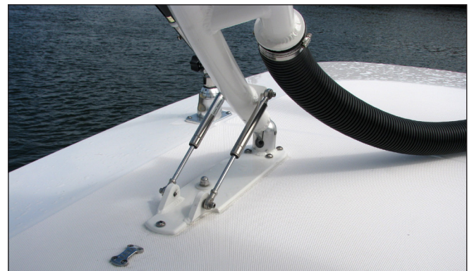
Gas Charged Assist Springs
