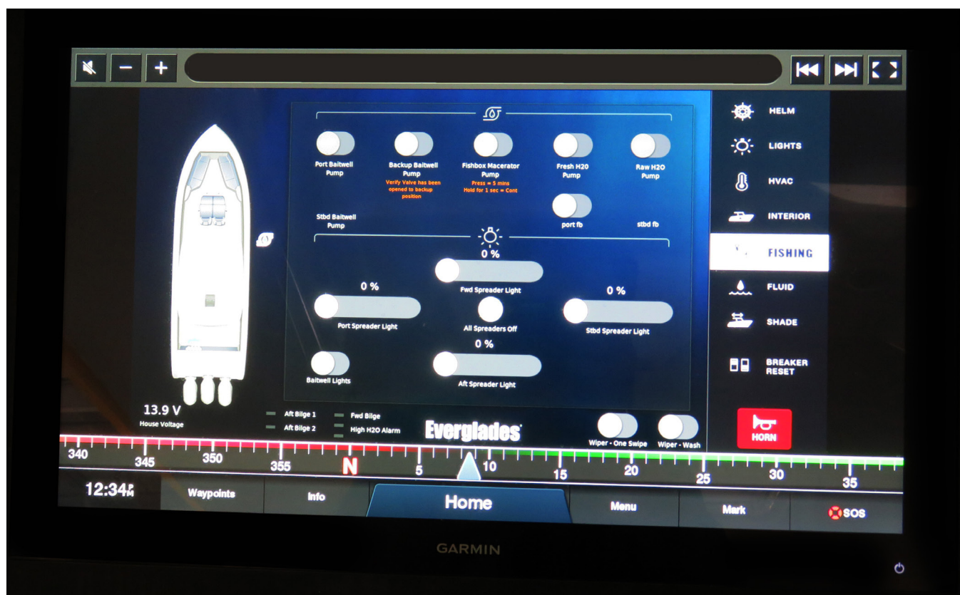
Typical Digital Switch Control Screen
