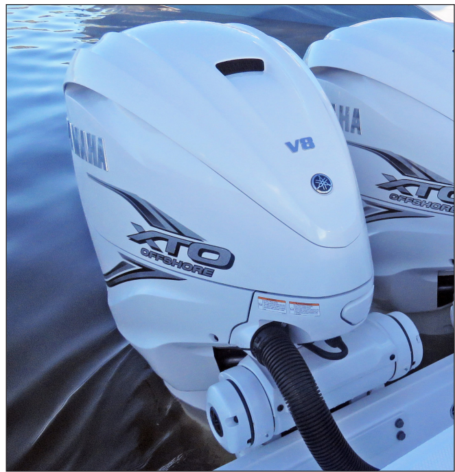
Helm Master Engine Mounted Electronic Steering
