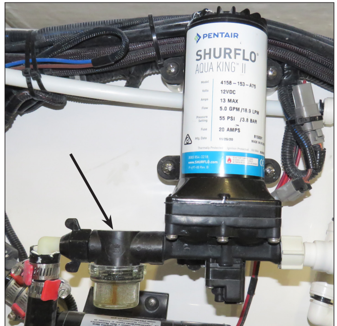
Raw Water Pump Strainer
