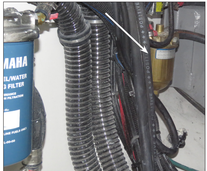
Diesel Fuel Filter
