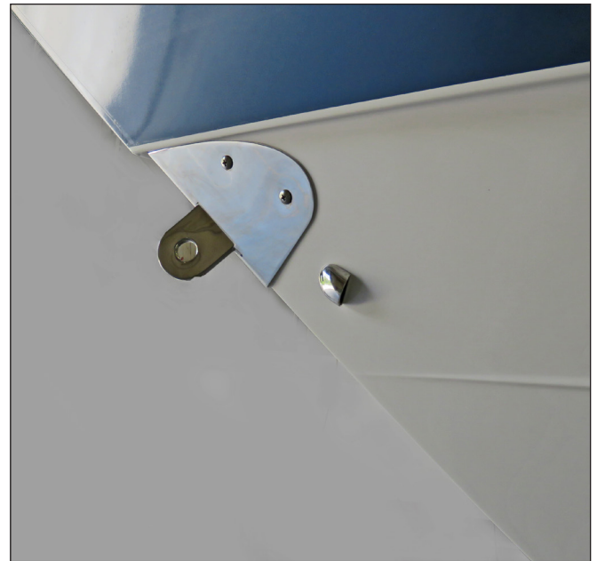
Typical Rope Locker Drain Fitting in Hull Side
