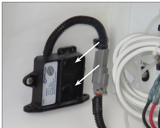
High Water Alarm Automatic Switch & Test Recesses
