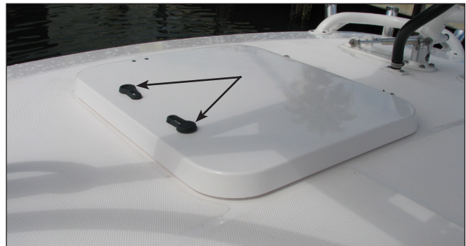
Upper Station Access Hatch Note exterior access hatch cam latch levers.
