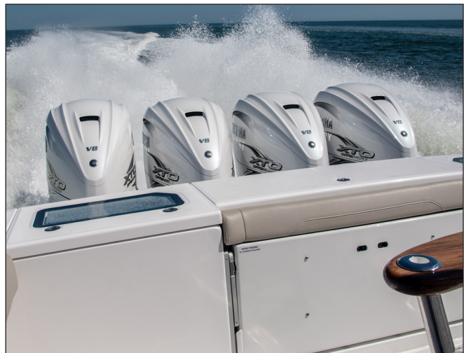
Typical Yamaha Quad Engines with Integrated Electronic Controlled Steering
