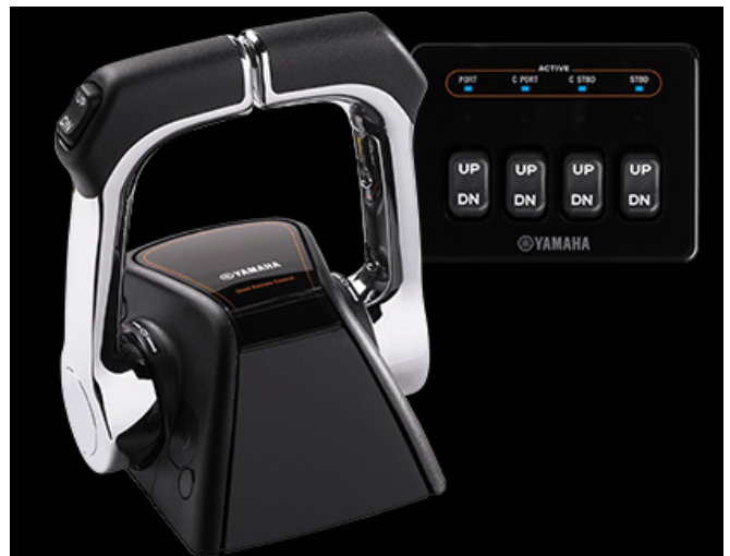
Yamaha Quad Engine DEC Control with Separate Trim Switches
