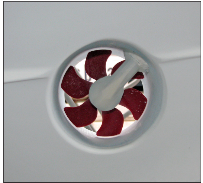
Typical Bow Thruster Drive Unit, propeller & tunnel
