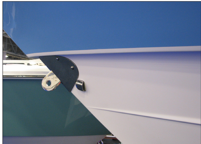
Rope Locker Drain Fitting in Hull Side
