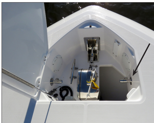
Fresh Water Washdown Faucet in Winch Compartment
