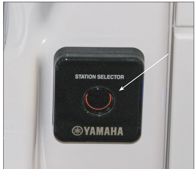
Typical Yamaha Triple Engine Station Transfer Button
