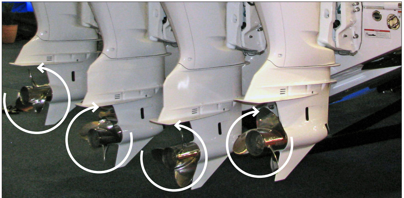
Typical Quad Engine & Propeller Rotation
