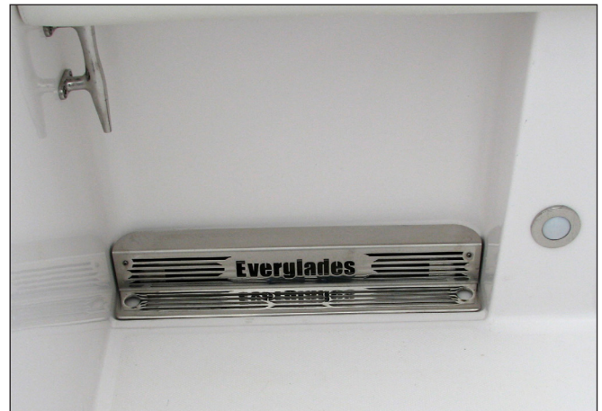
Typical Scupper Drains & Drain Rail
