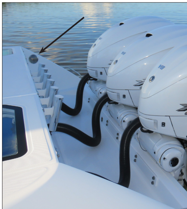
Starboard Bilge & Mechanical Systems Compartment Free Air/Forced Air Vent Aft of Cockpit
