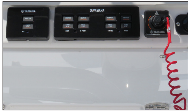
Yamaha Quad Engine Stop Switch & Lanyard Ignition START/STOP Switches
