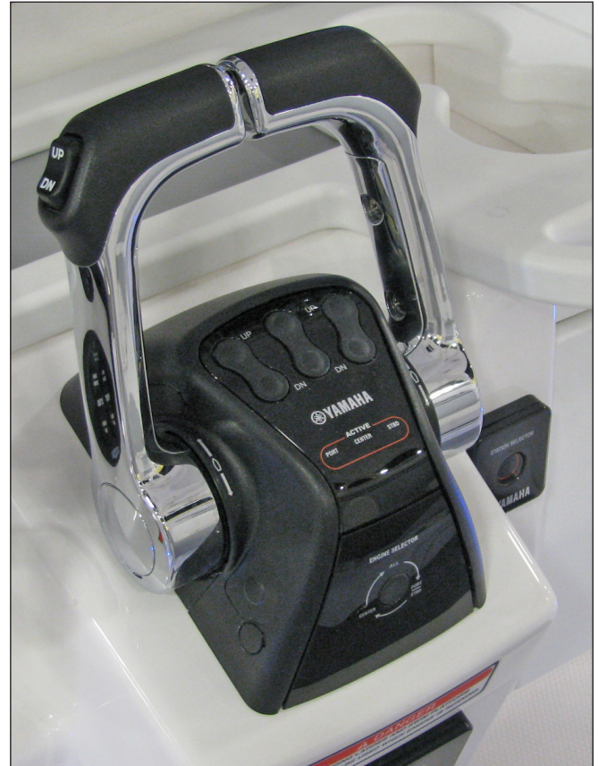
Typical Yamaha Triple Engine DEC Control
