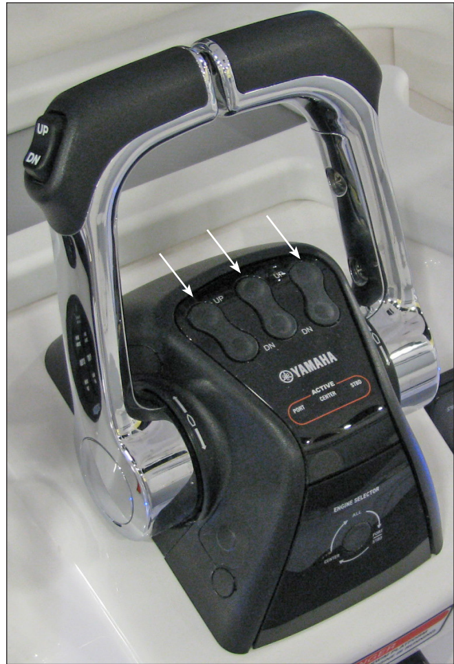
Yamaha Triple Engine DEC Control Trim Switches
