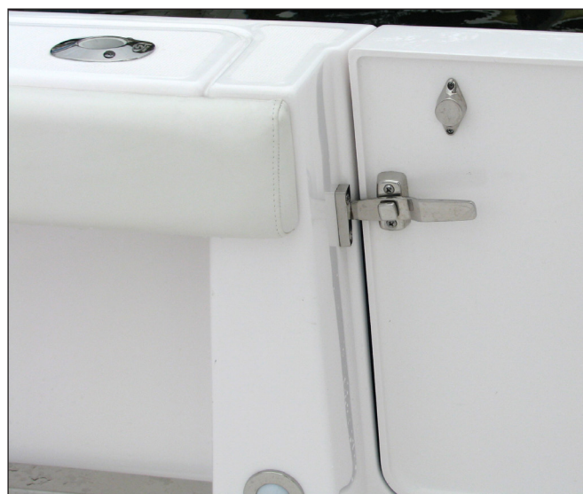
Side Door Main Latch & Spring Loaded Safety Pin
