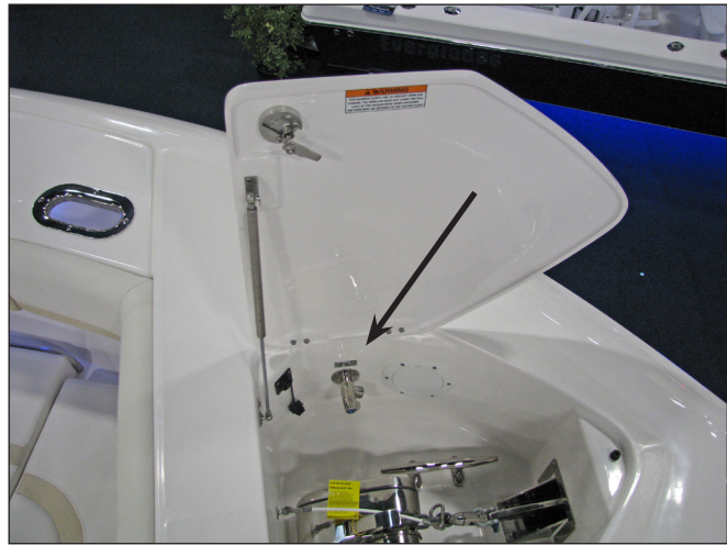
Windlass Raw Water Washdown Hose Connection
