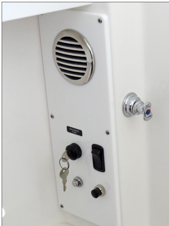
Head Switch Panel & Shower Control Valve
