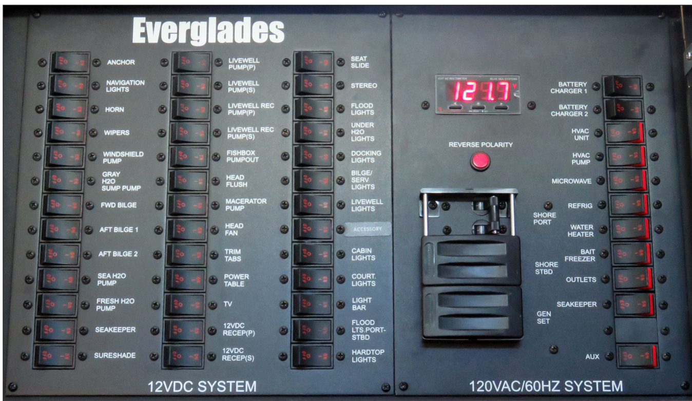
Cabin DC/AC Panel
