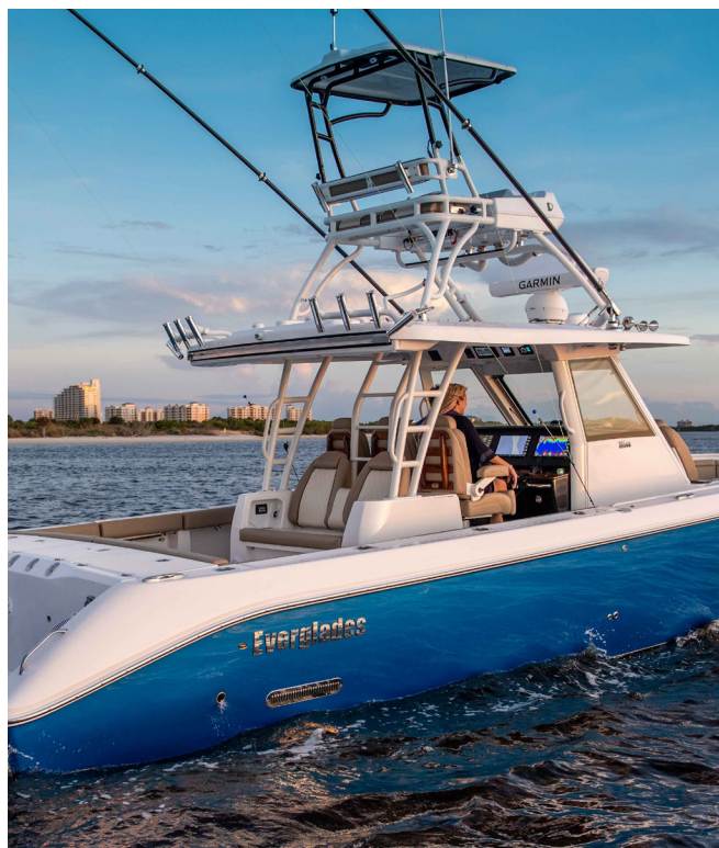
Upper Station Ladder, Mezzanine & Sunshade
