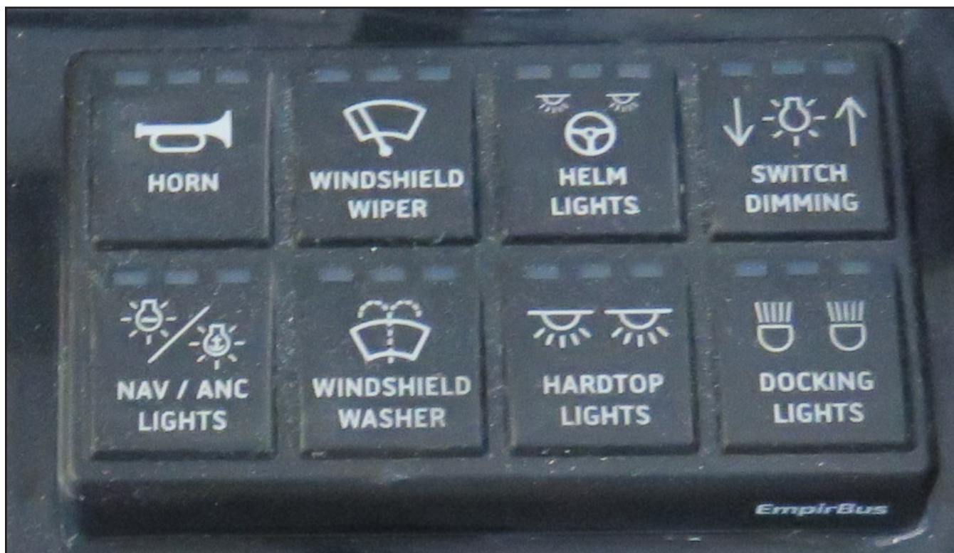
Helm Switch Panel on Starboard Side of Steering Wheel
