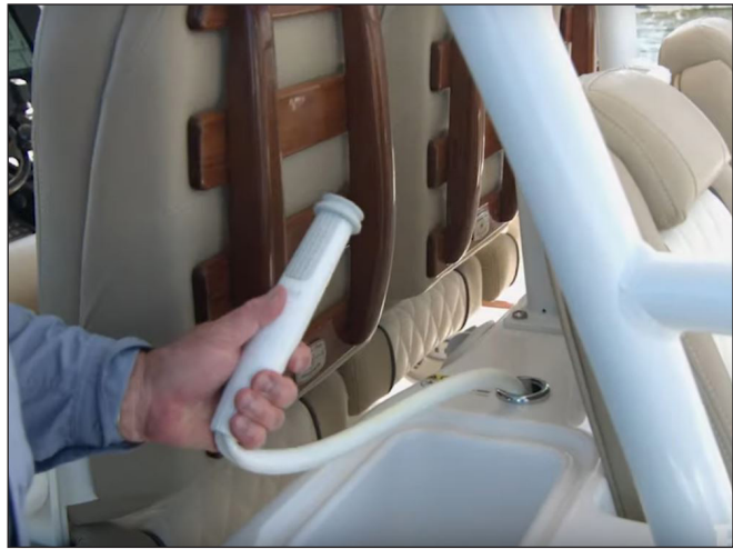
Cockpit Fresh Water Shower in Mezzanine
