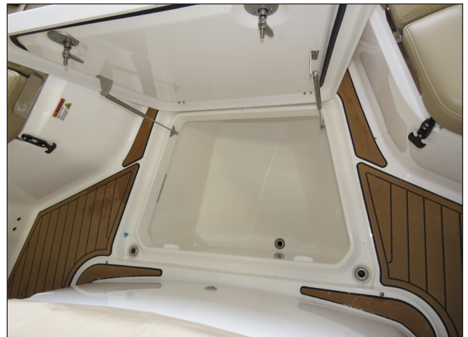
Forward Fishbox Drain & Drain Rails
