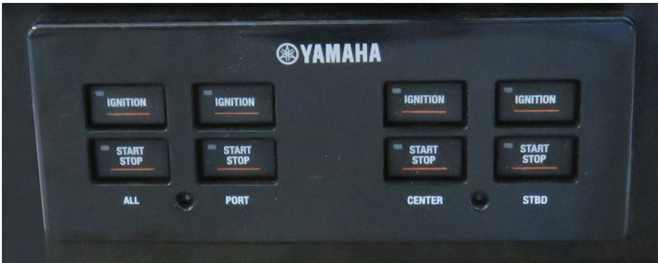
Typical Yamaha Helm Master Triple Engine Radio Frequency ID Key Activated START/STOP & Ignition Switch Panels
