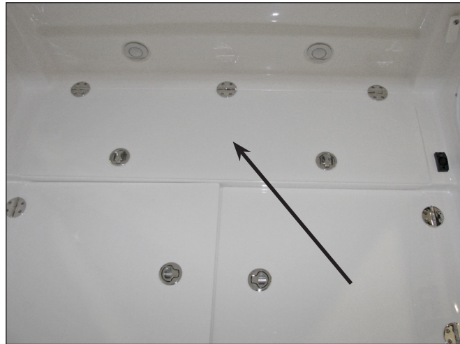
Removable Hatch to Access Back of Helm
