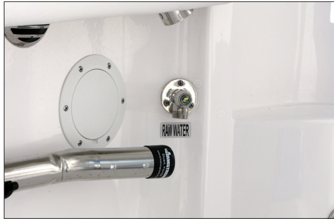
Typical Washdown Hose Connection
