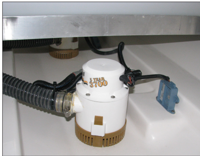
Typical Bilge Pump and Automatic Switch
