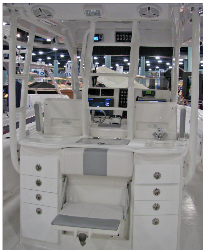
Upper Station Ladder and Work Station Showing Jump Seat and Work Station as Steps to the Ladder Note the Grab Rails on Each Side of Ladder
