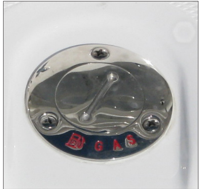
Typical Fuel Fill
