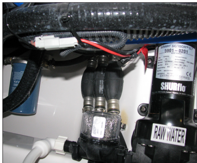
Primer Bulbs Near Fuel Filters
