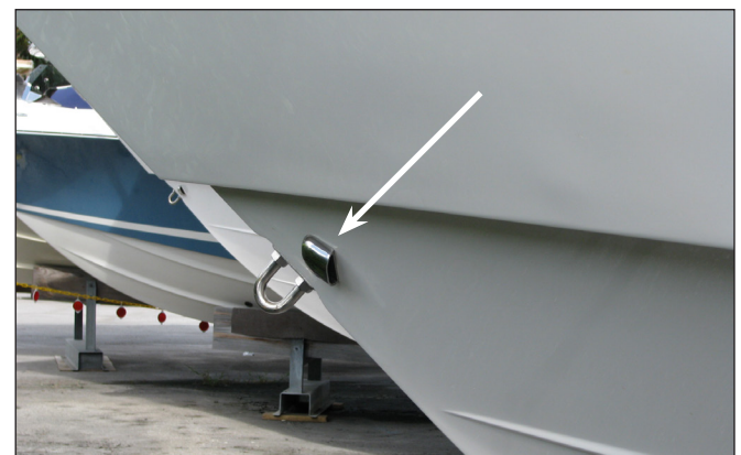
Rope Locker Drain Fitting in Hull Side
