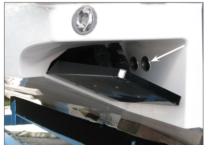
Scupper Drain Thru-hull Fittings
