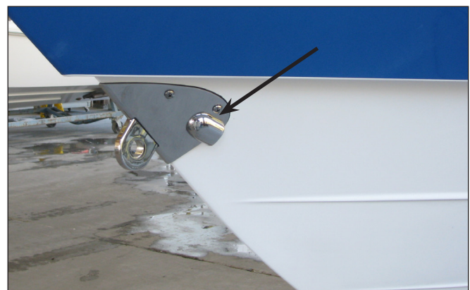
Rope Locker Drain Fitting in Hull Side
