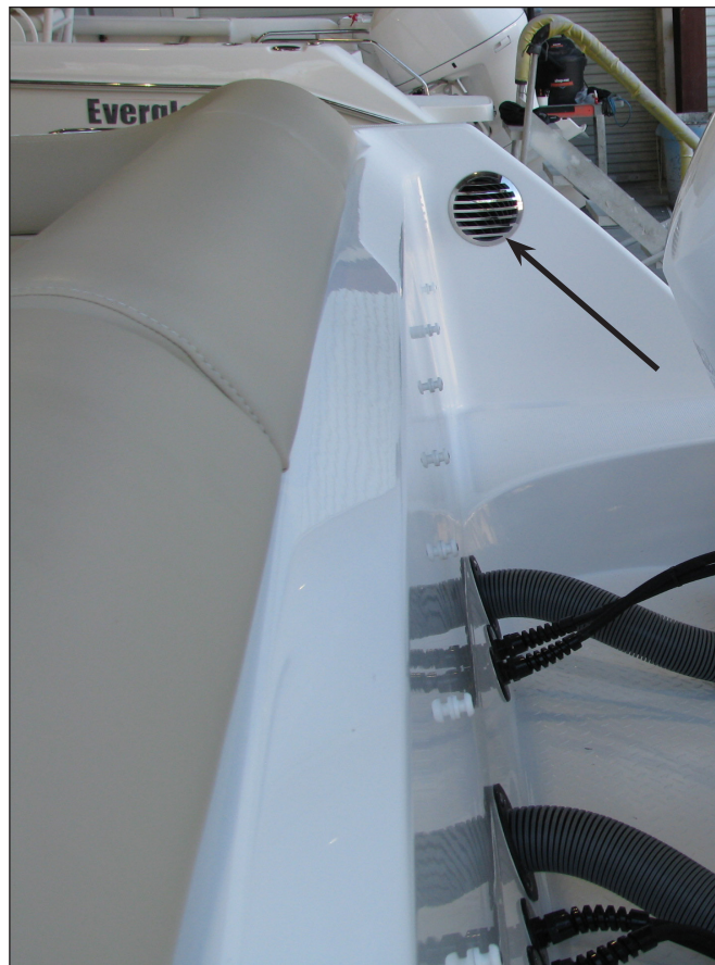
Aft Forced Air Vent
