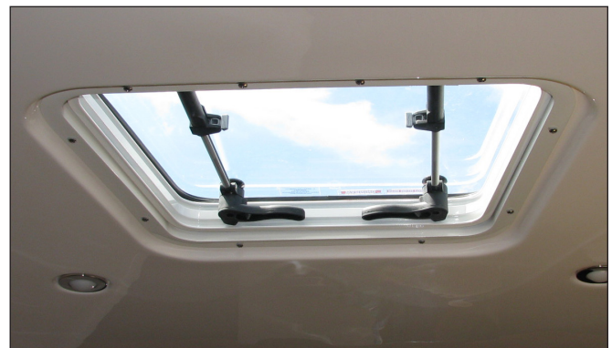
Deck Hatch Latched in the Vent Position
