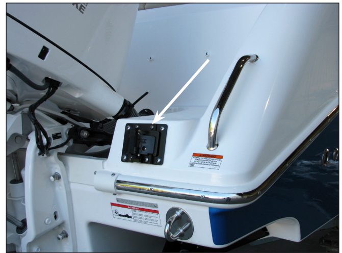
Ladder Retracted & Secured with Retaining Pin
