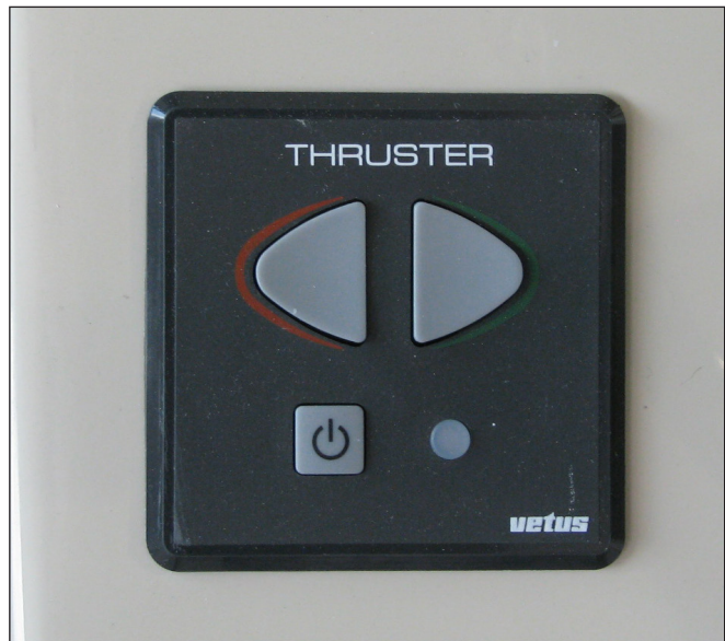
Bow Thruster Control Panel
