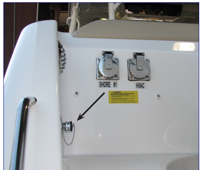
Shore Water Inlet Connection
