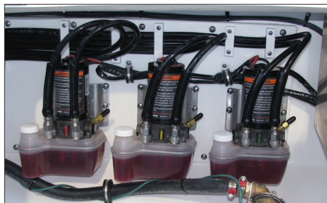
Independent Yamaha Electronic Steering Pumps
