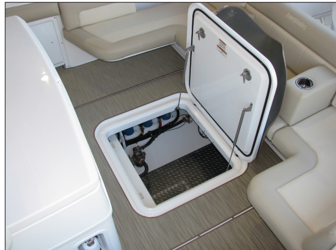
Systems Compartment Hatch
