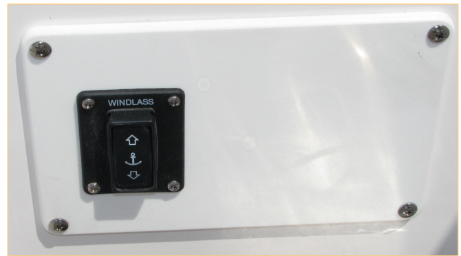
Windlass Switch in the Rope Locker
