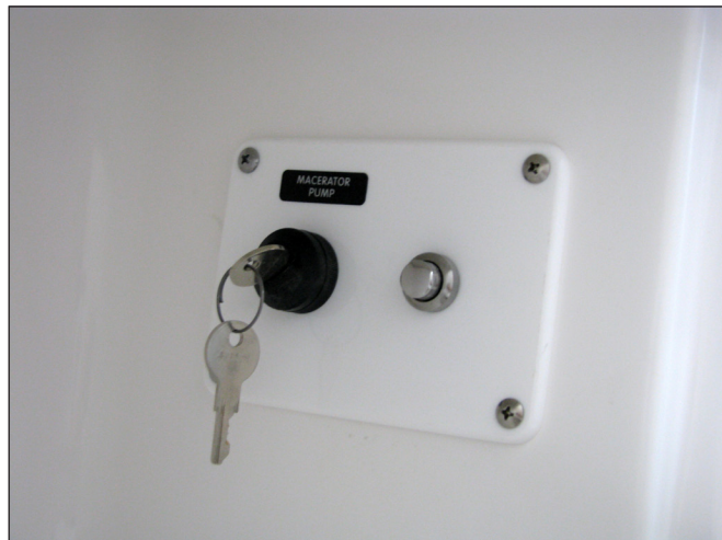
Macerator Discharge & Key Lockout Switches In Compartment Next to the Head
