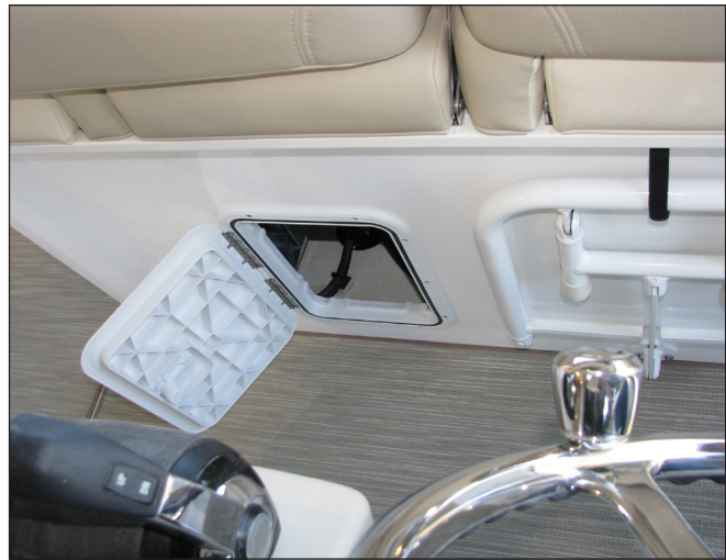
Prep Island Equipment Access Hatch
