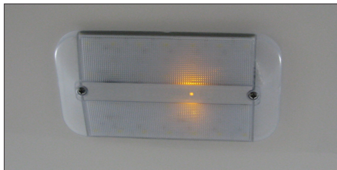
Aft System Compartment Light W/ Touch Activated Switch
