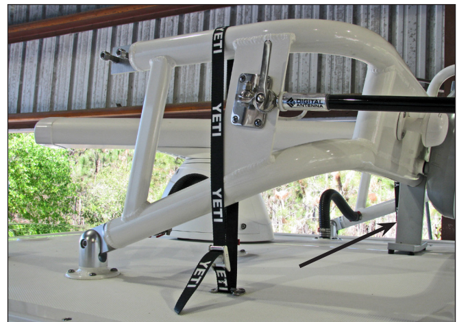
Radar Arch Folded & Secured to Hardtop & Arch Support
