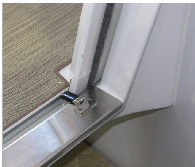
Cabin Door Latched in Open Position
