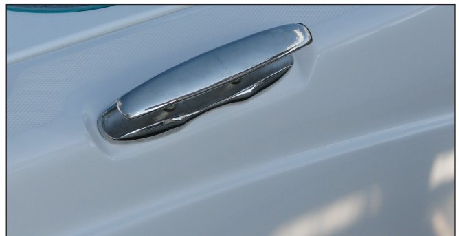
Typical Cleat in the Mooring Position
