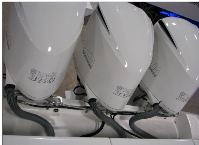
Tie Bars and Dual Steering Cylinders Typical Triple Engine Steering Shown
