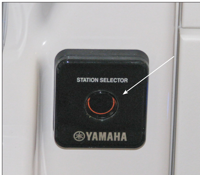
Typical Yamaha Station Transfer Button
