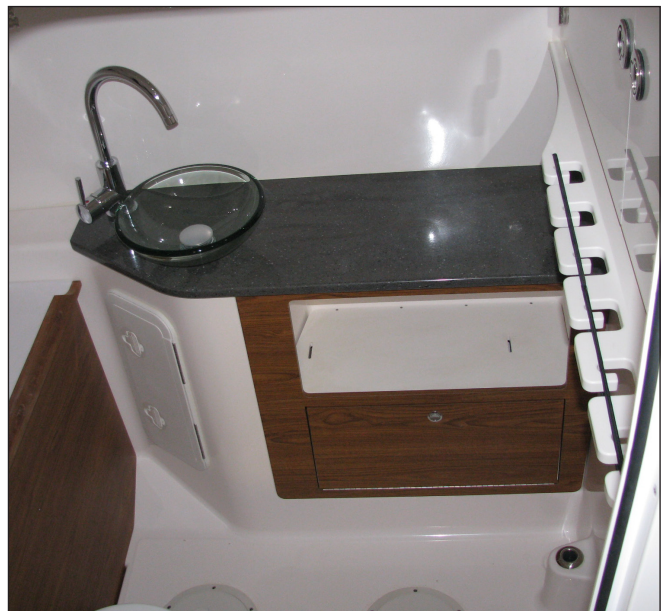
Head Compartment Vanity Sink and Faucet
