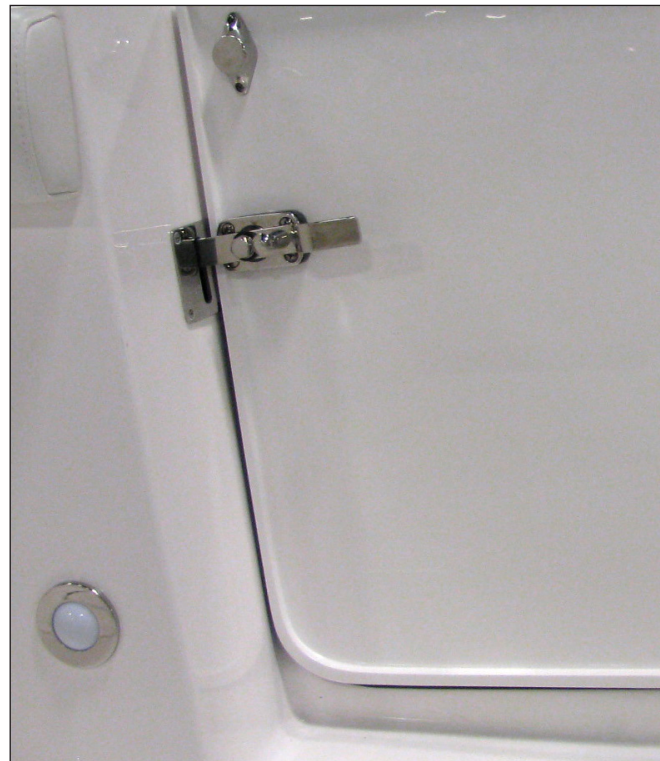
Utility Door Latch and Safety Pin
