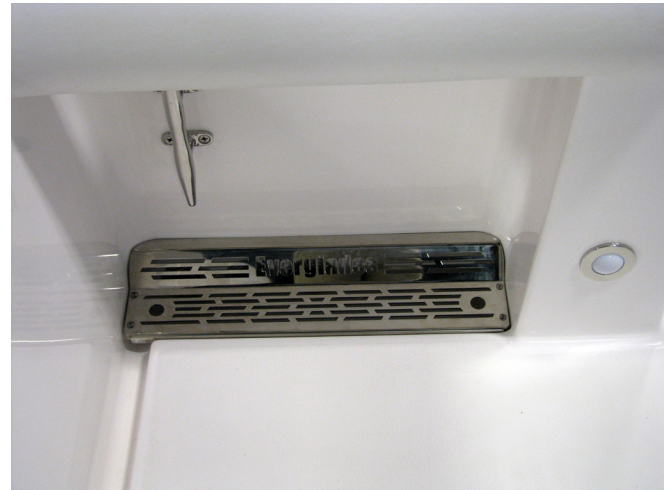
Typical Cockpit Scupper Drain and Drain Rail
