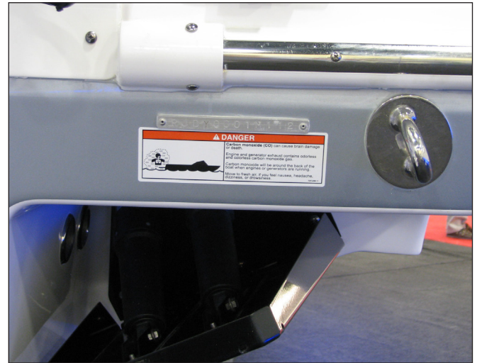
Hull ID # On Starboard Side of Transom
