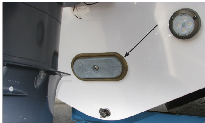
Typical Transom Anode
