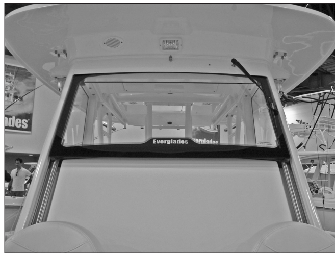
Sliding Windshield, Windshield Wiper & Washer
