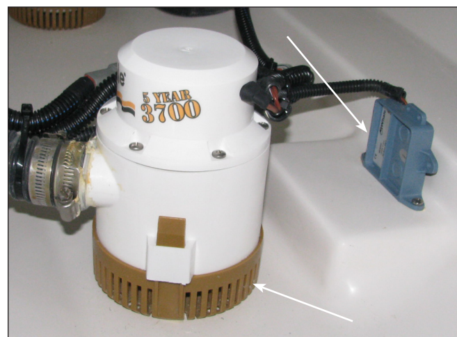
Bilge Pump Strainer and Automatic Switch
