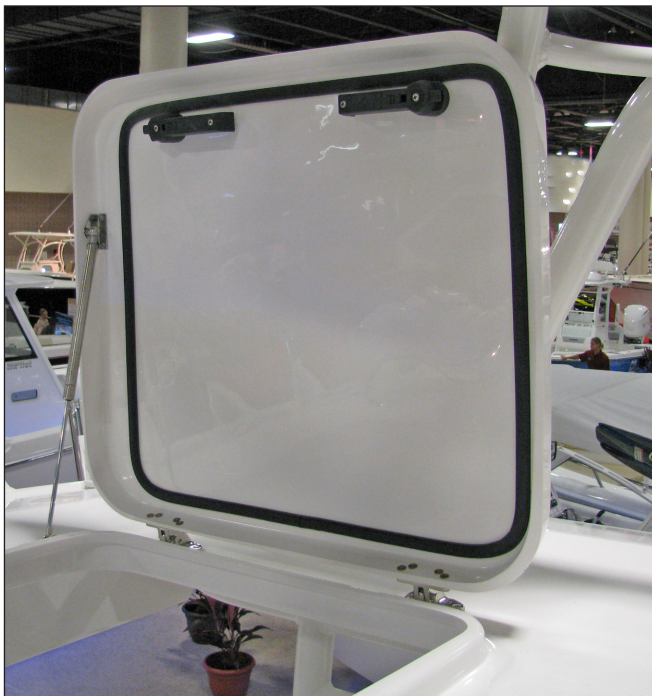
Upper Station Access Hatch Twist Action Cam Levers
