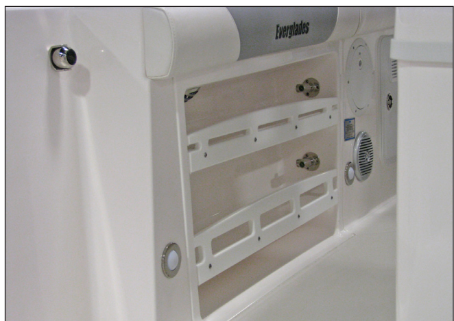
Freshwater & Raw Water Washdown Connections
