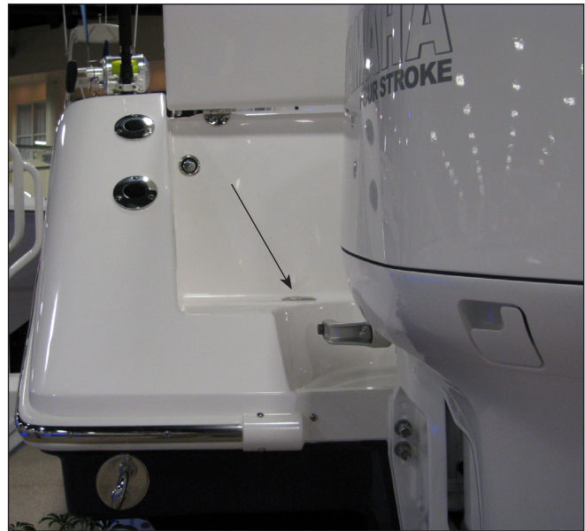
Port Splashwell Platform and Water Tank Fill
