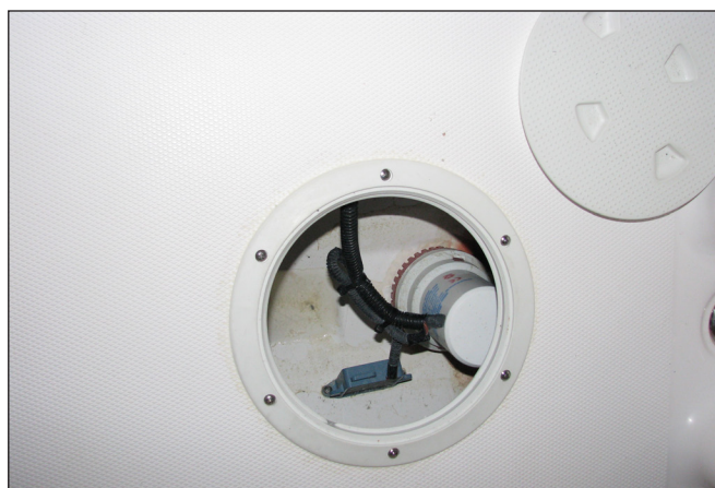
Forward Bilge Pump and Automatic Switch
