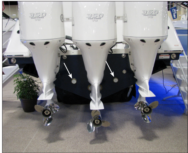
Engine Mounting System and Underwater LED Lights
