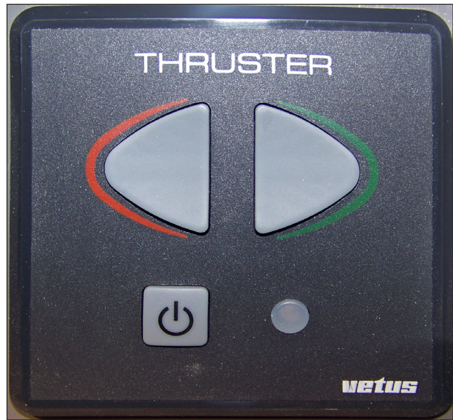
Typical Bow Thruster Control Touch Pad
