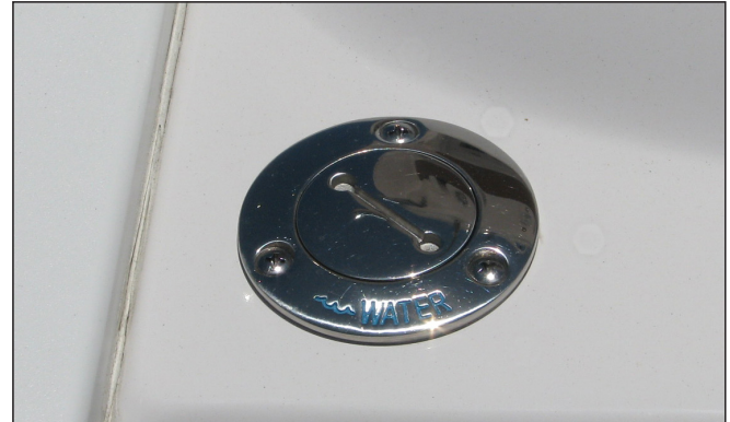
Fresh Water Fill
