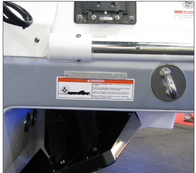
Hull ID # On Starboard Side of Transom
