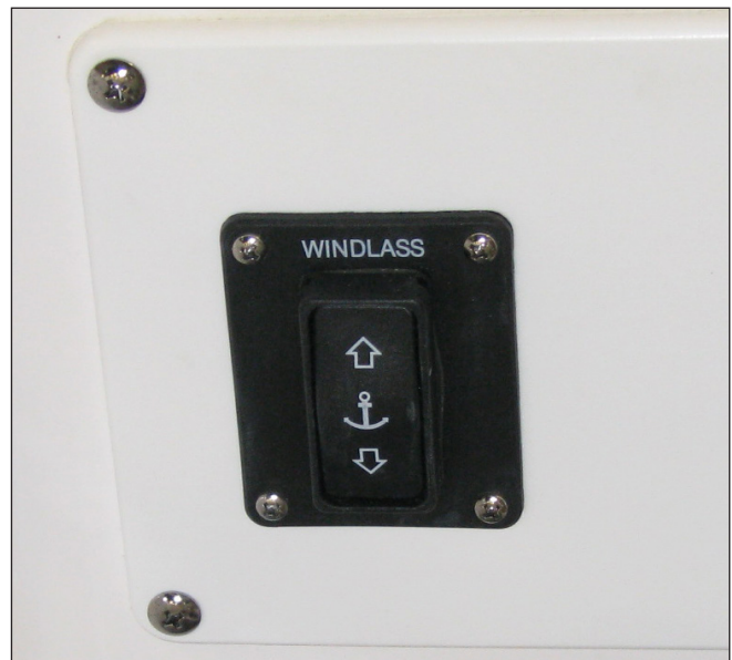
Windlass Switch in Rope Locker Near Windlass
