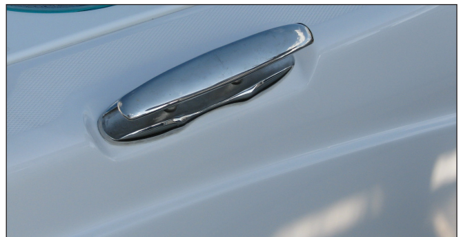
Typical Cleat in the Mooring Position
