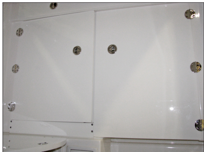
Access Doors to Compartments for Electronics Modules, accessory Circuit Breaker Panel and Opening Helm Latches
