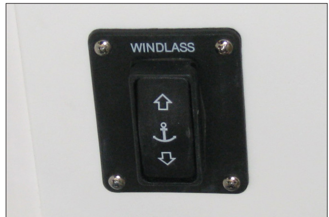
Windlass Switch in the Rear of the Rope Locker
