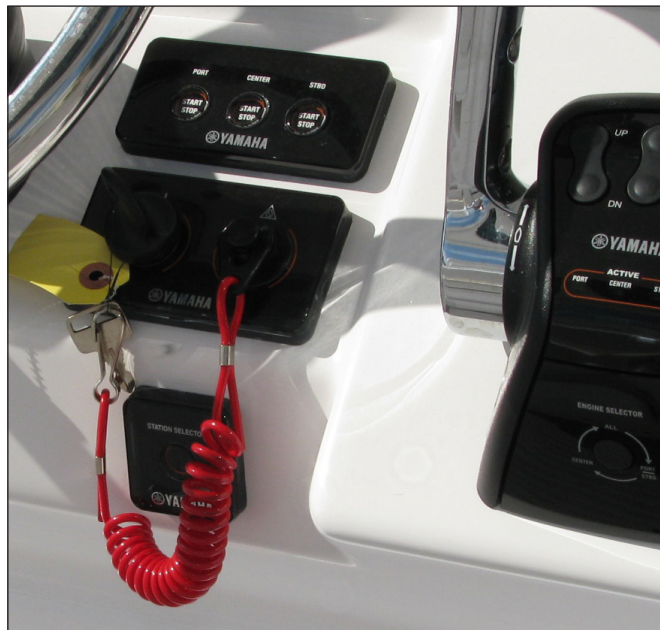
Engine Stop Switch & Lanyard Ignition Switch
