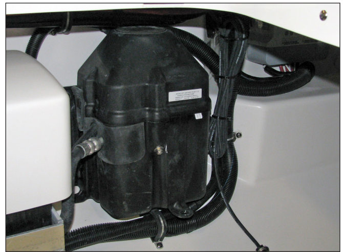
Power Steering Unit in the Systems Compartment
