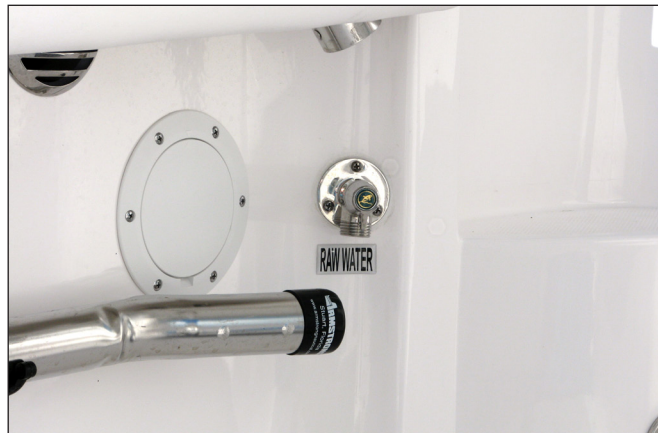
Typical Washdown Hose Connection
