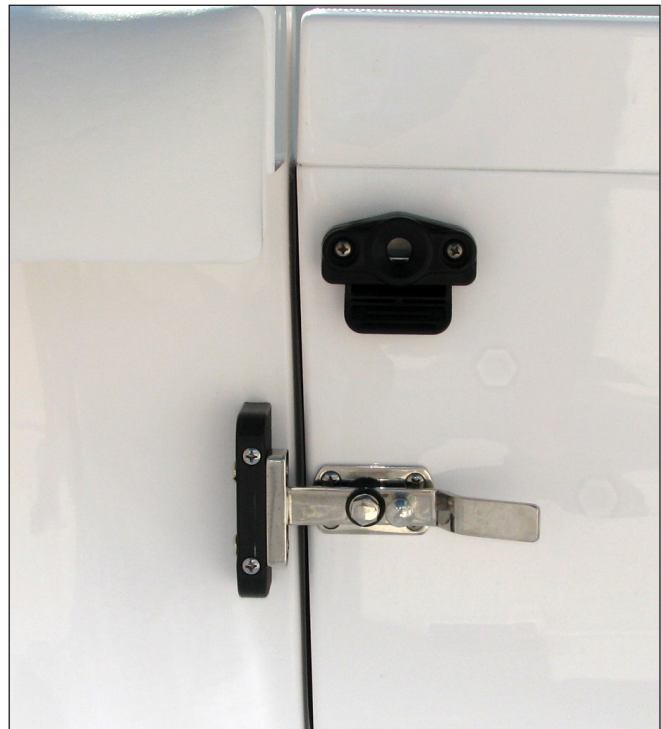
Dive Door Latch and Safety Pin
