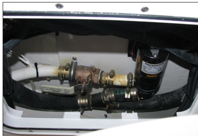
Macerator Pump and Discharge Valve
