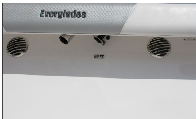
Bilge and Systems Compartment Vents
