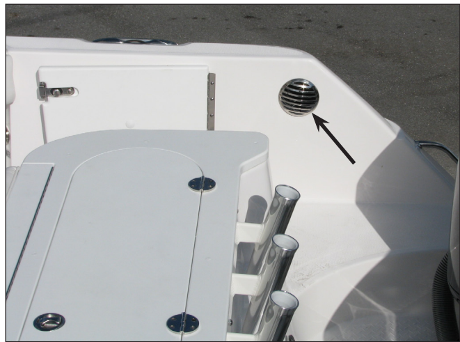
Aft Forced Air Vent
