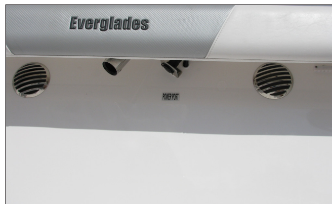
Bilge and Systems Compartment Vents
