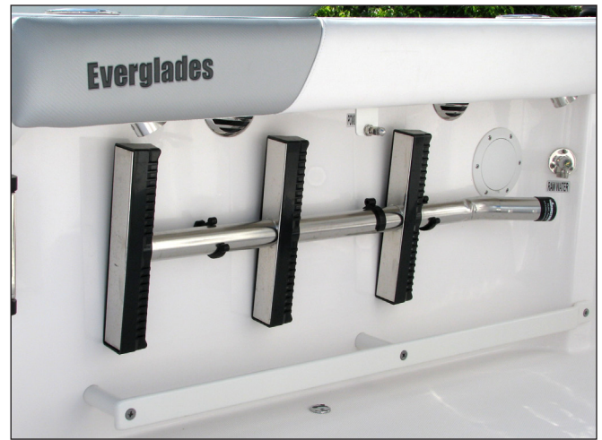
Dive Ladder in Storage Brackets
