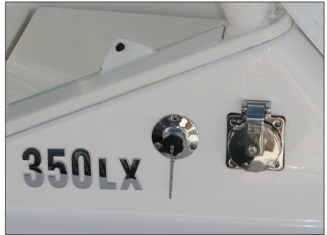
Shore Power Inlet Plug and Shore Water Connection
