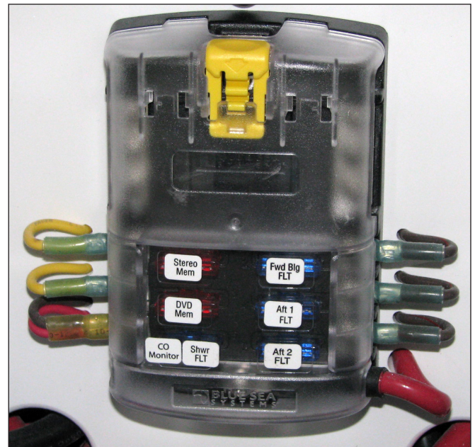
Continuous Power Fuse Panel
