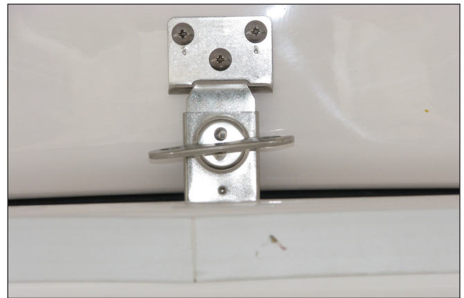
Rotating Draw Latch on Overhead Electronics Locker
