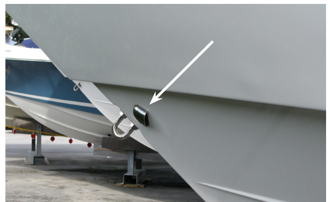
Rope Locker Drain Fitting in Hull Side
