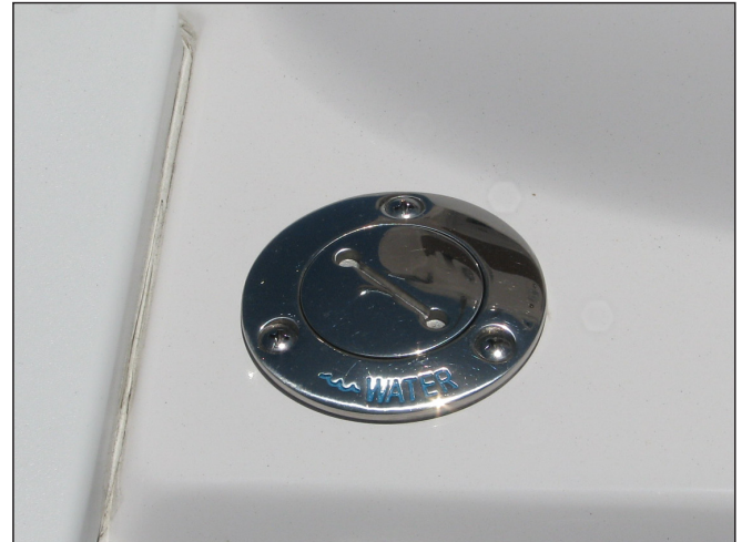
Fresh Water Fill
