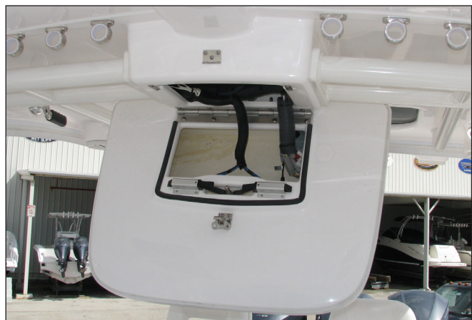
Overhead Electronics Locker Lowered for Inside Access
