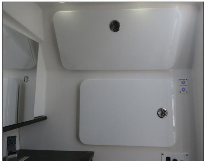
Access Hatches in Rear Bulkhead
