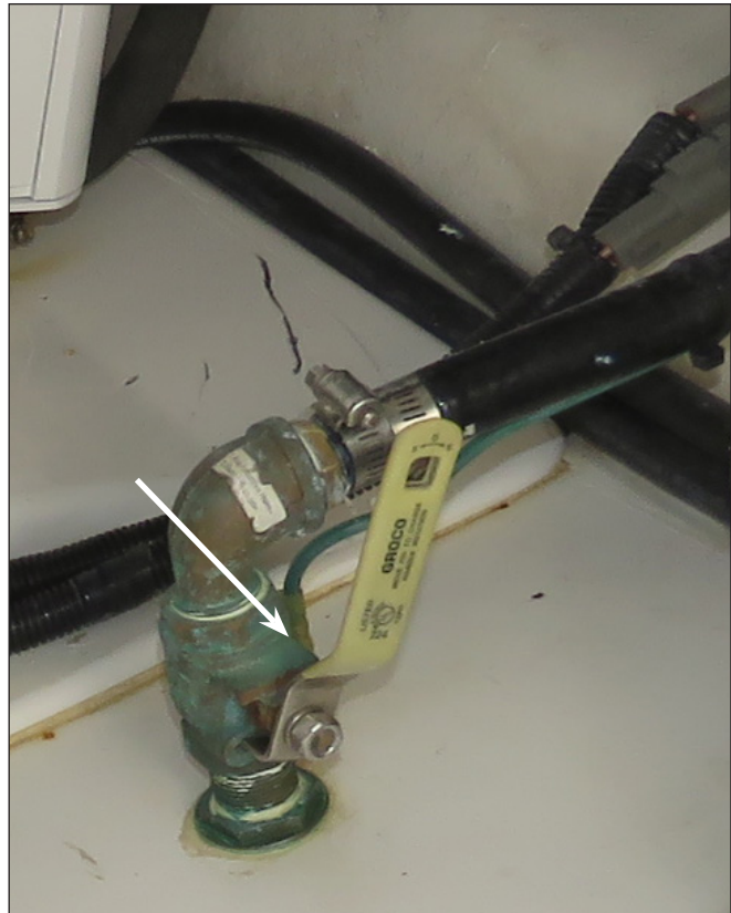
Typical Seacock Bonding Wire & Connection
