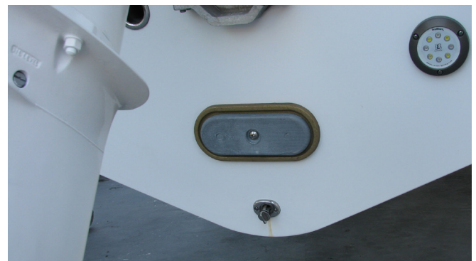
Typical Transom Anode
