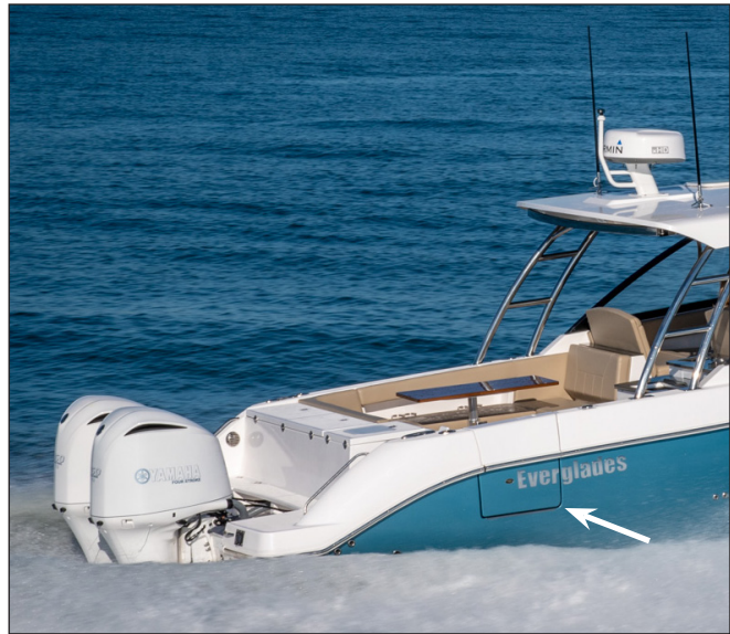
Side Utility Door
