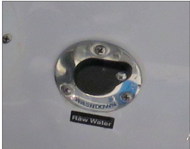
Raw Water Washdown Connection
