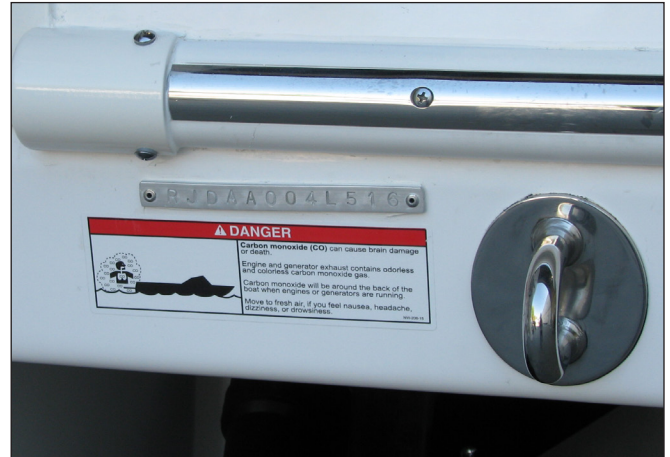
Hull ID # On Starboard Side of Transom
