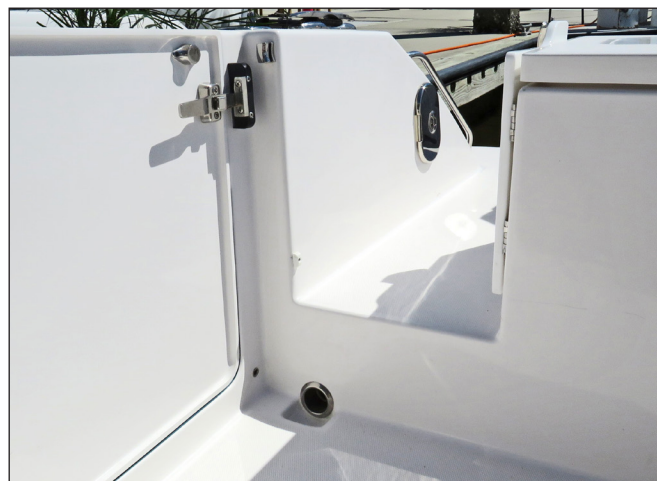
Typical Scupper Drains
