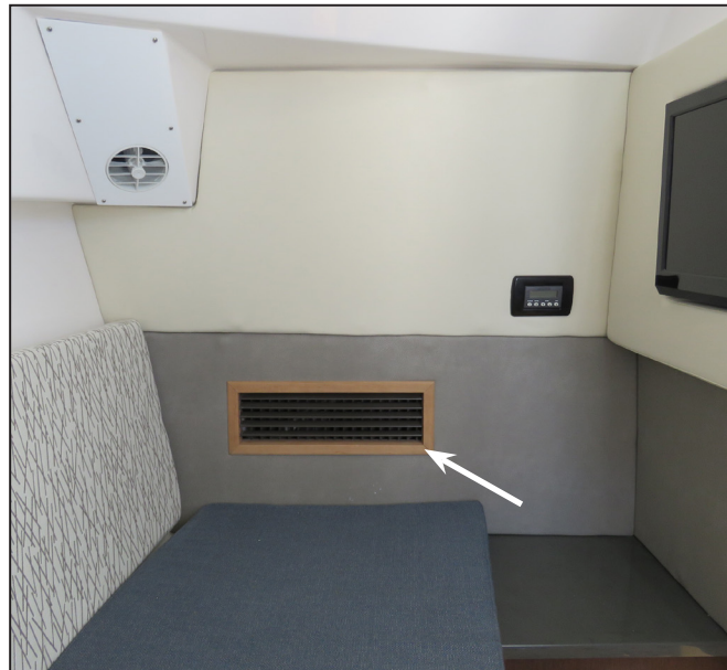
Air Condition Intake Vent
