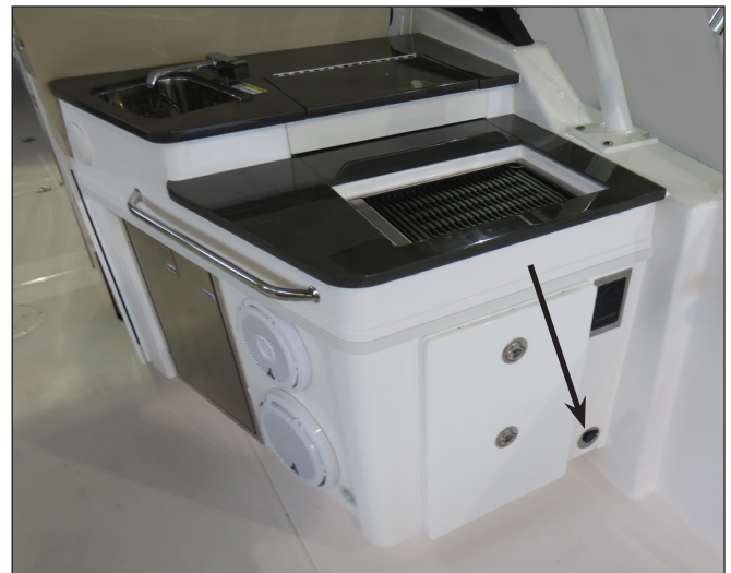
Fresh Water Washdown
