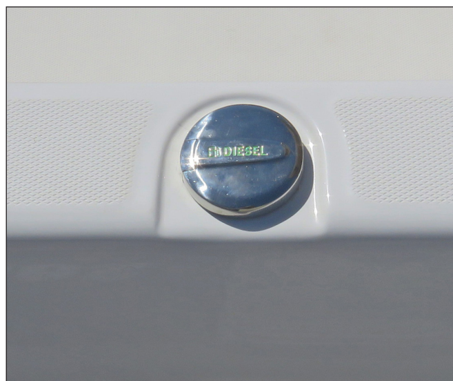
Diesel Fuel Fill
