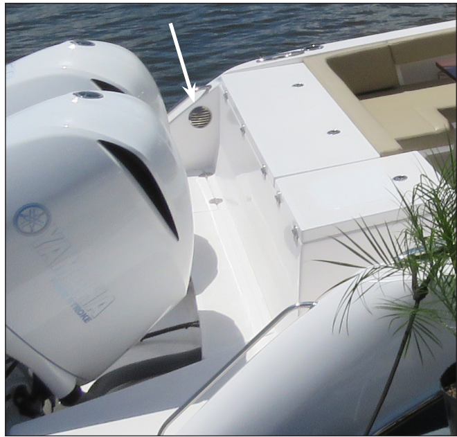
Bilge Free Air & Forced Air Vent
