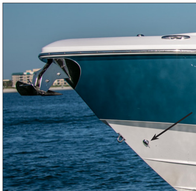
Rope Locker Drain Fitting in Hull Side
