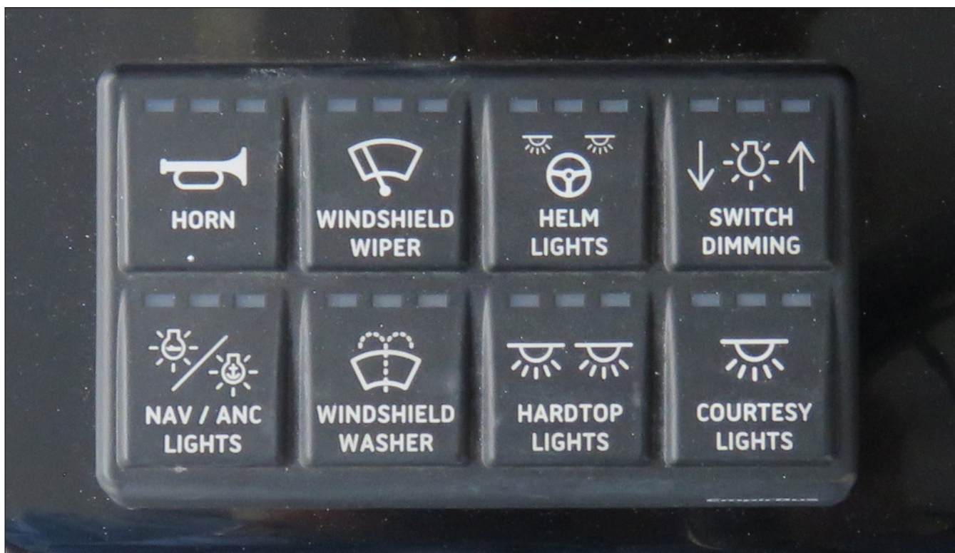
Helm Switch Panel On Port Side Of Steering Wheel
