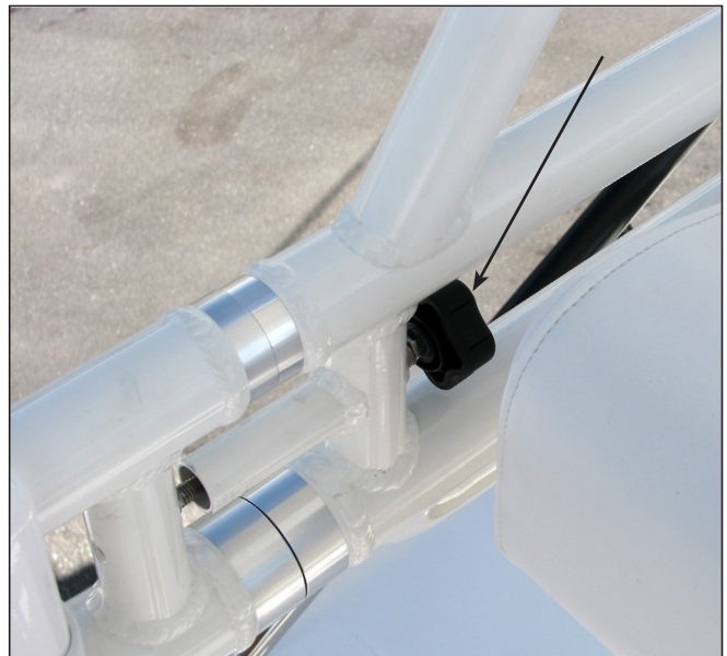
Hand Bolt On Each Side Securing Upper Station Sections
