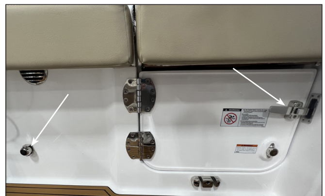
Side Boarding Door and Gate Closed Magnetic Latch & Door Latch w/ Safety Pin
