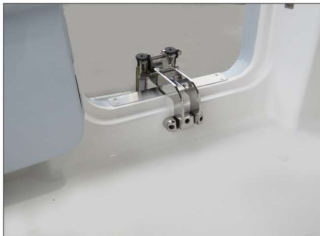
Ladder Secured To Side Door Bracket
