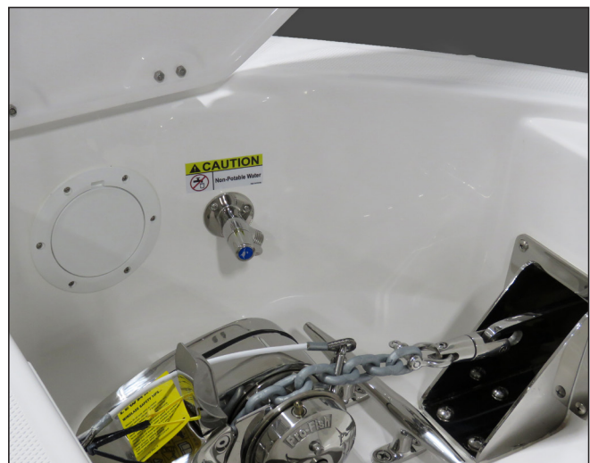
Windlass Compartment Washdown Connection
