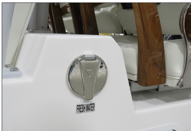
Fresh Water Shower/Washdown On Helm Seat Base
