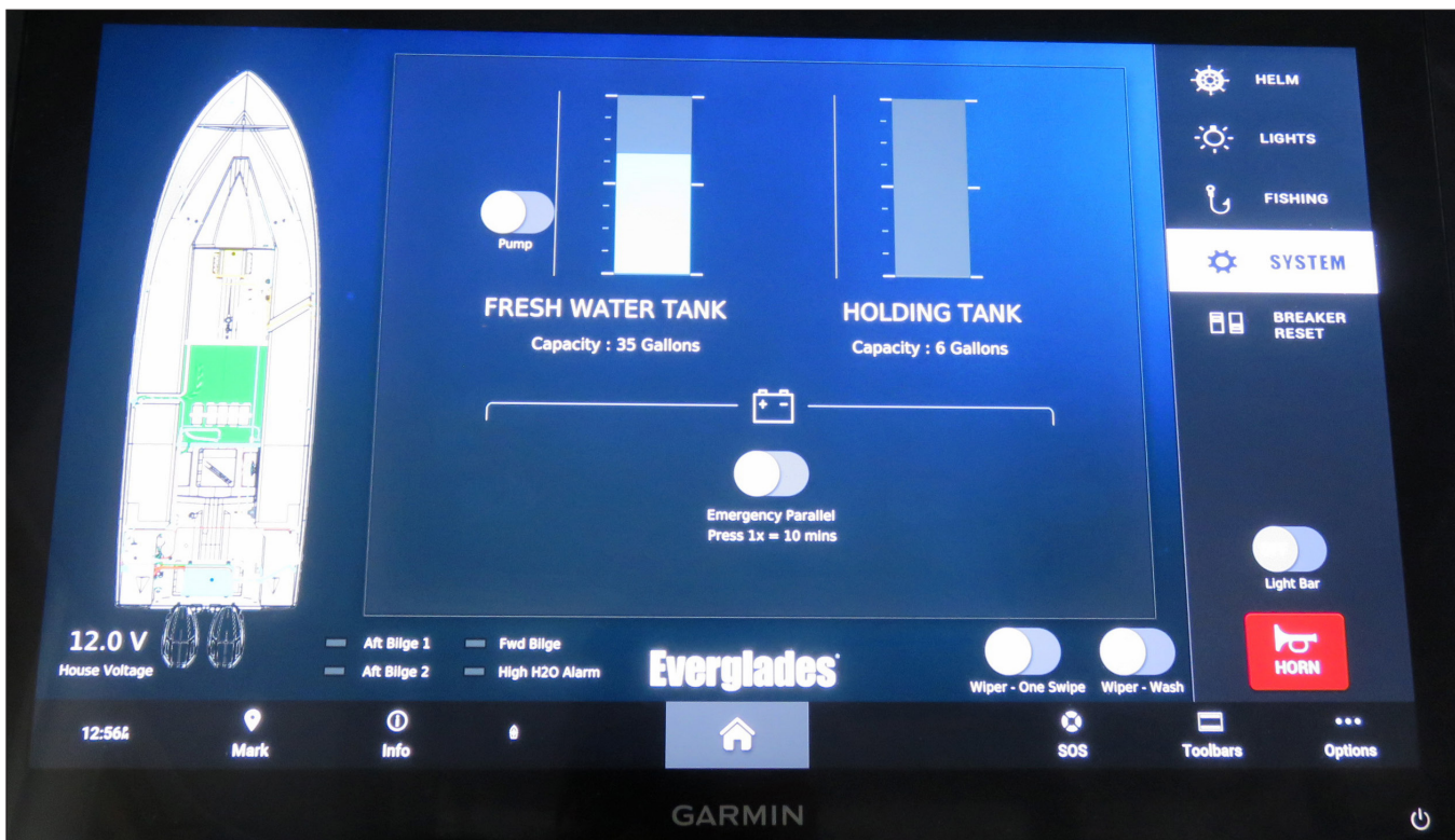
Typical Fluid Level Monitoring Screen
