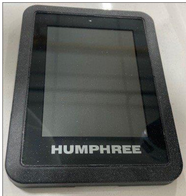
Trim Tab Control Panel
