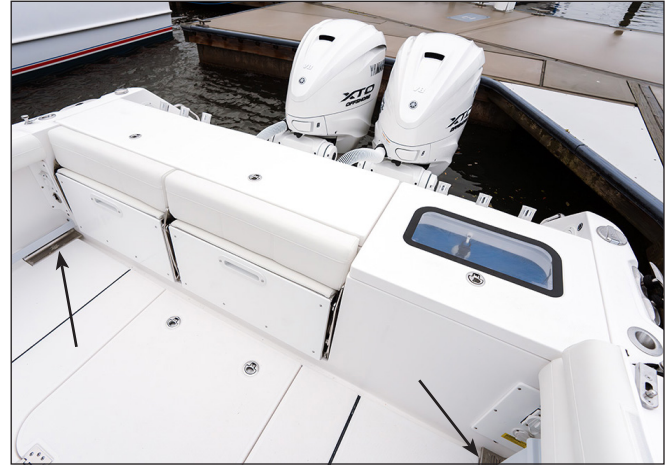
Typical Scupper Drains & Drain Rails
