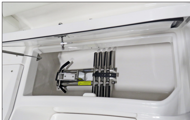
Ladder Secured In Starboard Bow Storage Compartment
