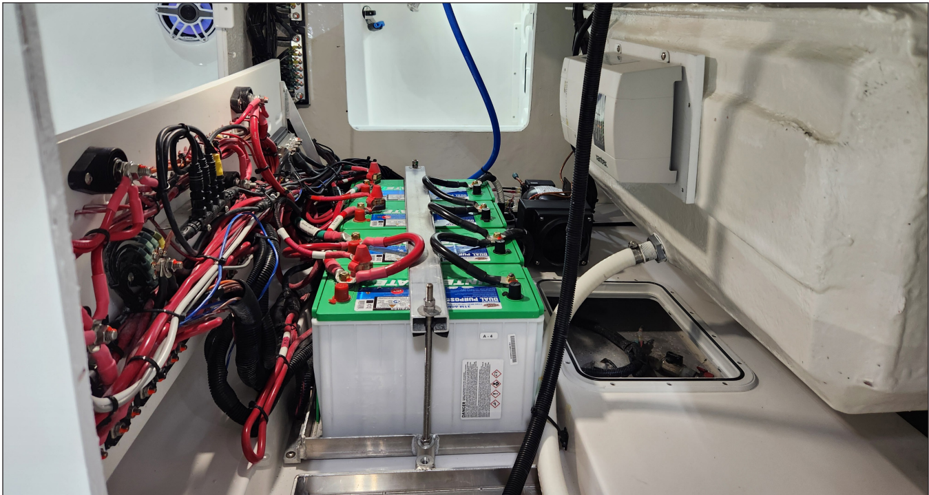
House & Engine Batteries In Compartment Below Helm Seats
