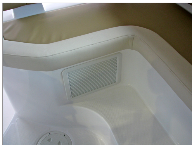
Helm Air Conditioning Air Intake
