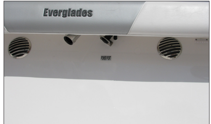
Bilge and Systems Compartment Vents
