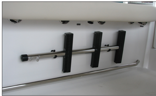
Dive Ladder in Storage Brackets
