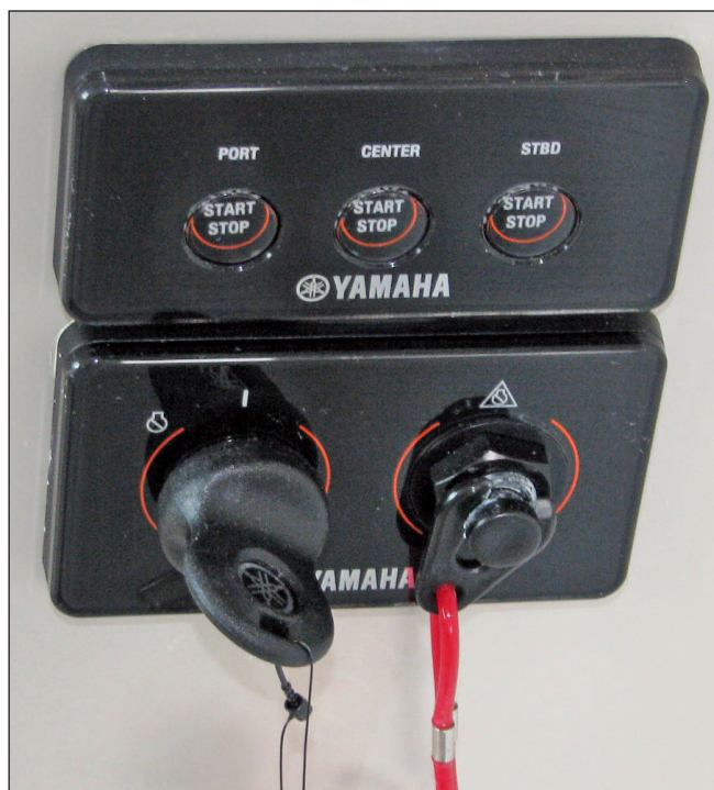
Typical Yamaha Triple Engine Ignition Switch, Start Buttons and Emergency Stop Switch
