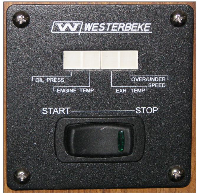
Cabin Generator Control Switch and Monitoring Lights
