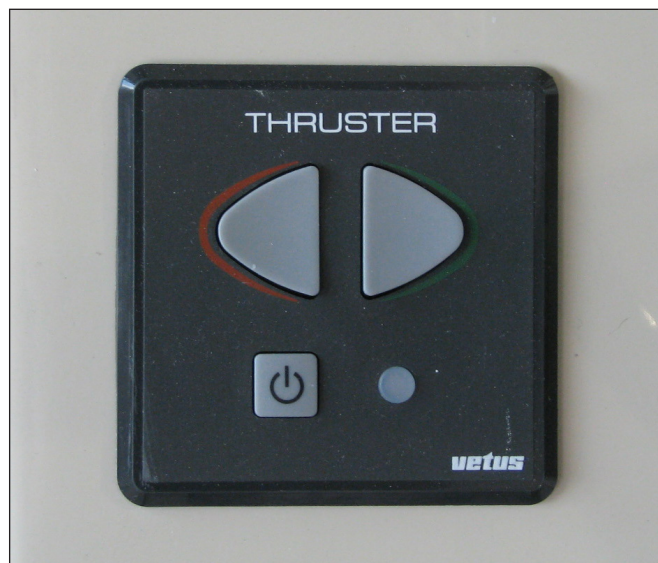
Typical Bow Thruster Control Panel
