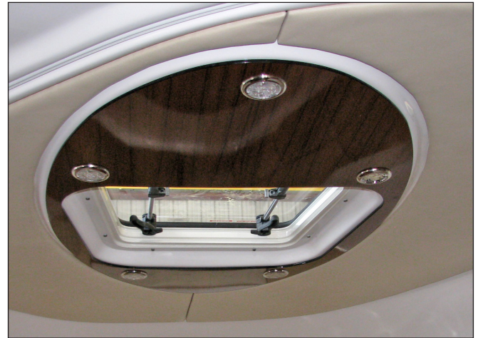
Typical Deck Hatch Latched in the Vent Position
