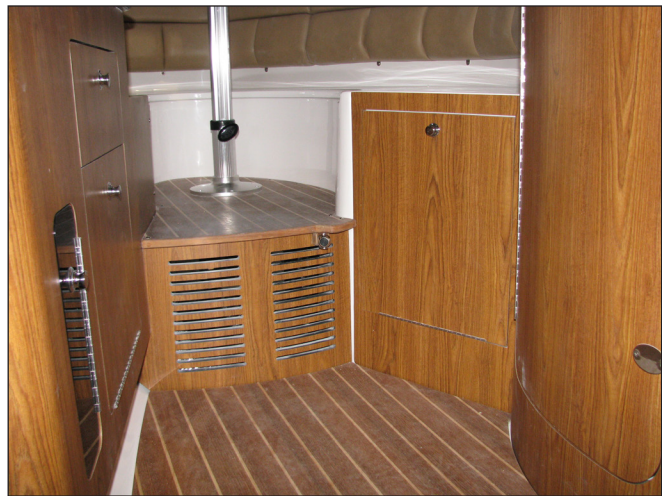
Air Conditioner in Compartment Below Table Pedestal
