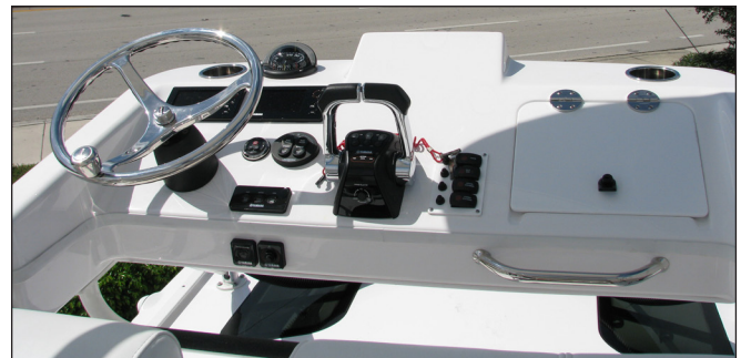
Typical Upper Control Station Helm
