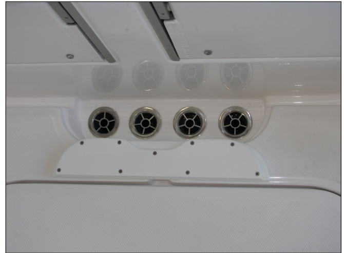
Typical Scupper Drains and Drain Rail
