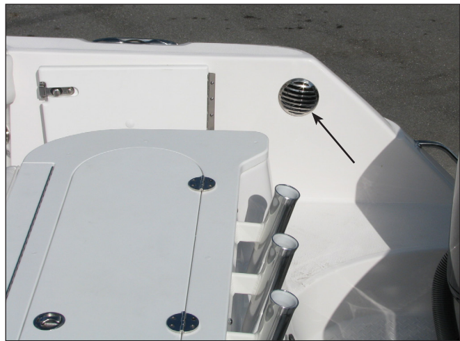
Aft Forced Air Vent
