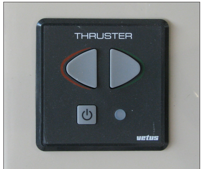
Typical Bow Thruster Control Panel
