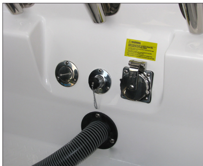
Shore Power Inlet Plug, Shore Water Connection and Fresh Water Tank Fill Fitting
