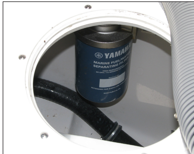
295 Pilot Fuel Filters Below Splashwell
