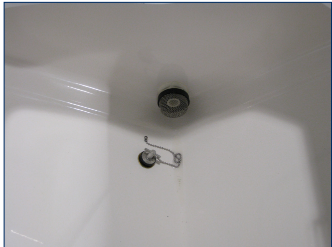
295 Pilot Forward Fishbox Pump out Strainer and Manual Drain Plug
