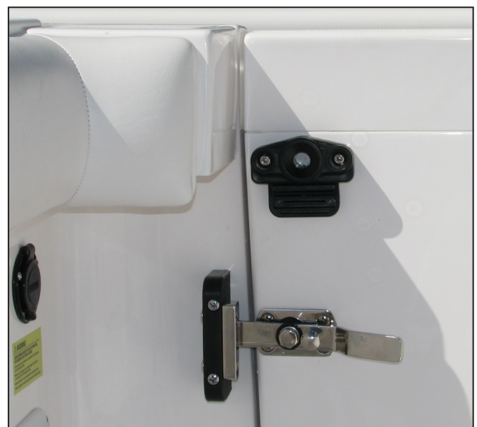
325 Pilot Utility Door Latch and Safety Pin
