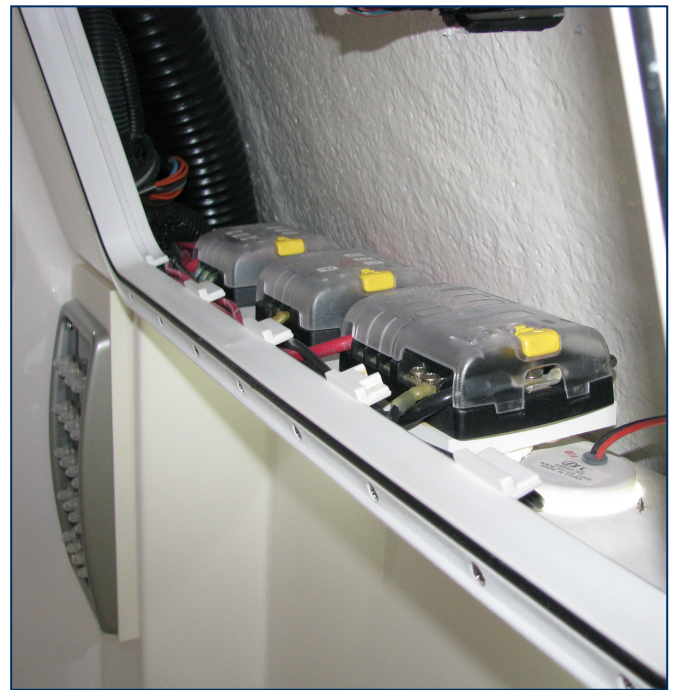
325 Pilot Typical Electronics and Accessory Fuse Panels
