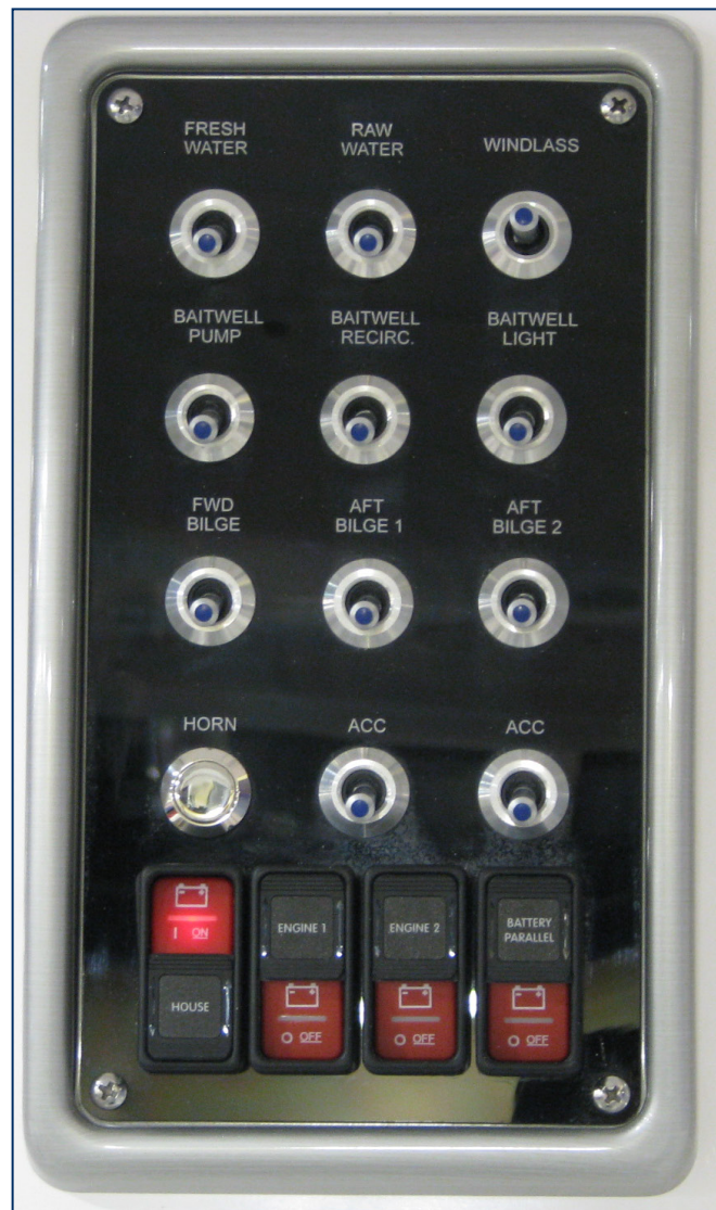
Remote Battery Switches House Switch in ON Position Engine and Parallel Switches in OFF Position
