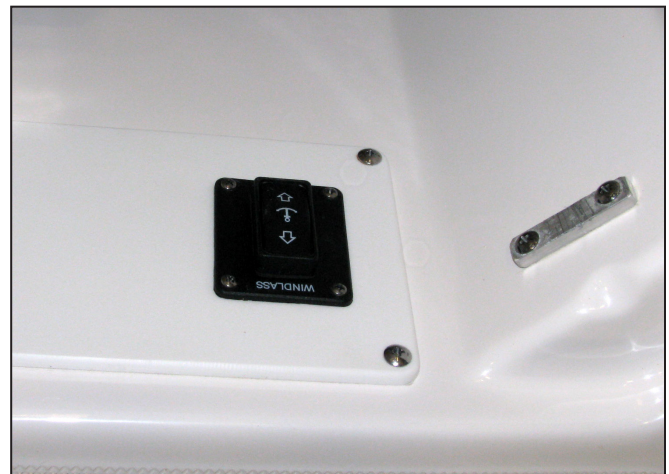
Windlass Switch in Windlass Compartment
