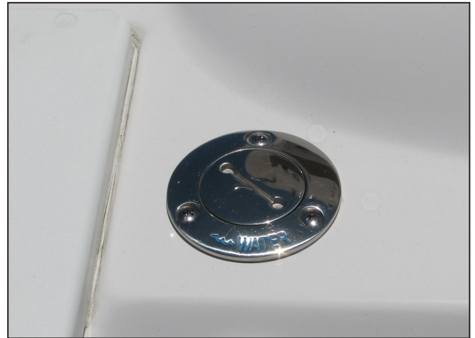
Fresh Water Fill
