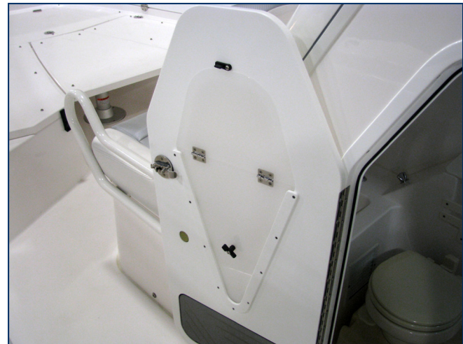
Head Compartment Door Vent Panel Open
