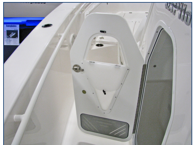
Head Compartment Door Vent Panel Closed Cabin Door Vent Twist Action Latches
