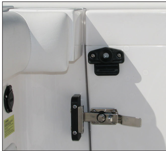
295 Pilot utility door Latch and Safety Pin
