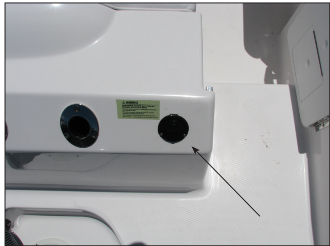
295 Pilot Shore Power Inlet Connection
