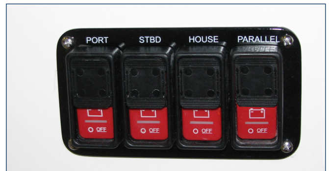
Twin Engine Remote Battery Switches
