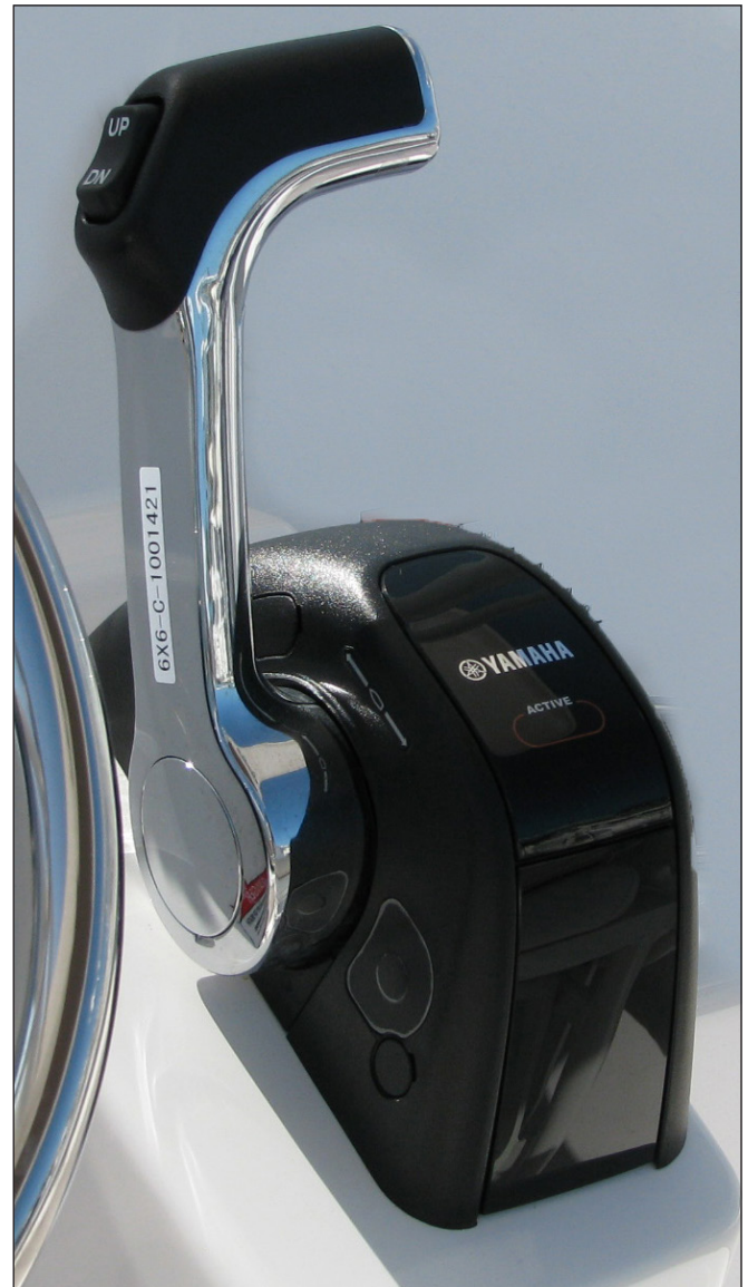
Typical Yamaha Single Engine Electronic Control
