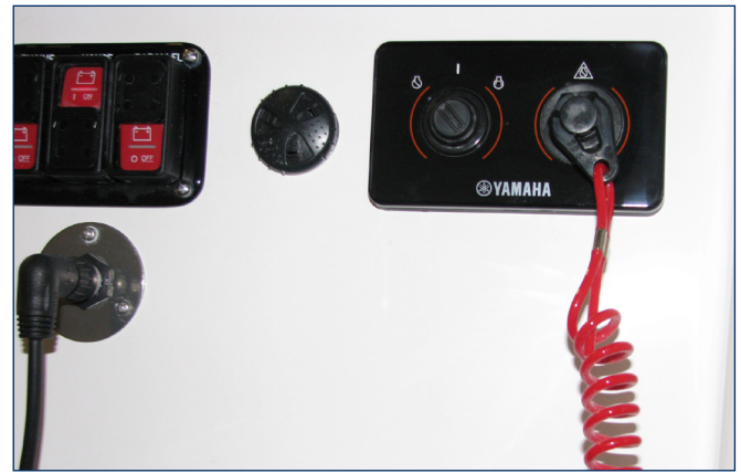
Typical Single Engine Stop Switch
