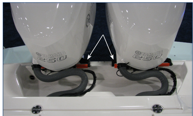
Electronic Steering System Cylinders
