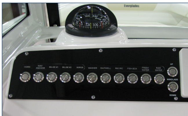
Port Side Helm Switches
