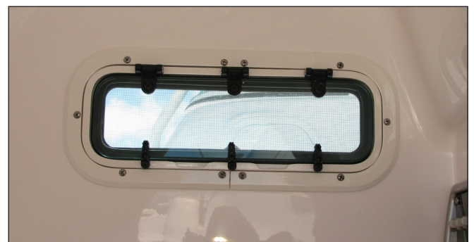
Cabin Port Window & Twist Action Locks
