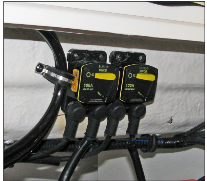
Typical Yamaha Engine Charging Circuit Protection
