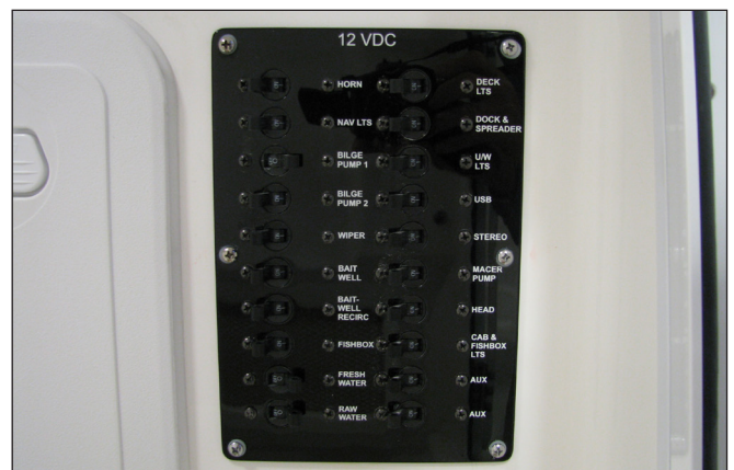
12 Volt Accessory Circuit Breakers
