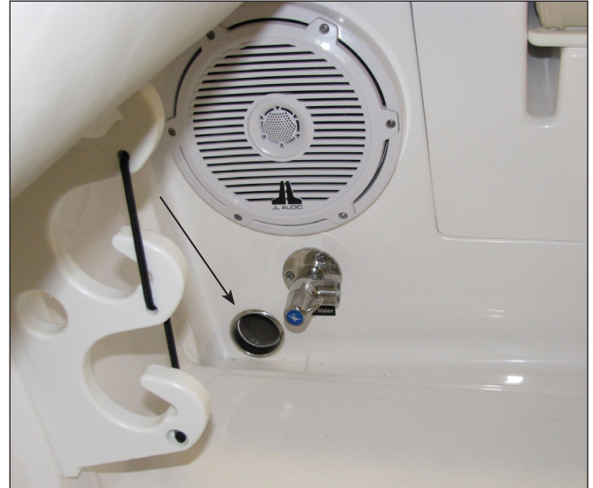
Cockpit Scupper Drain
