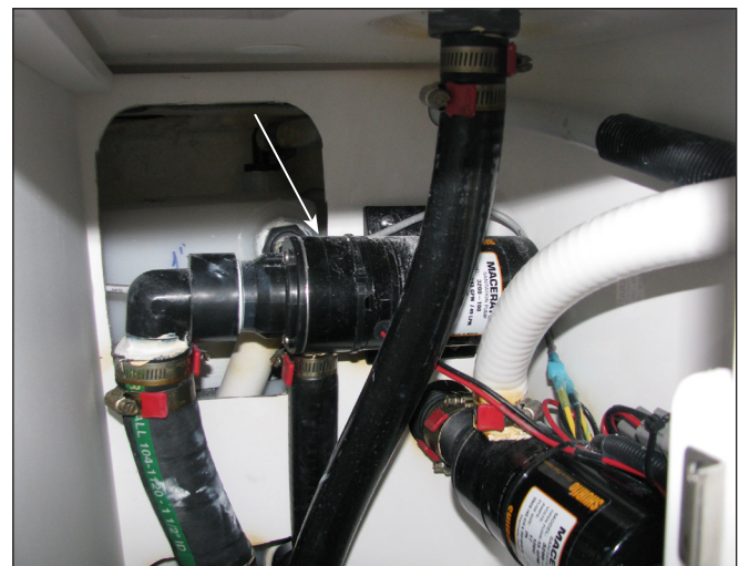
Forward Fishbox Pump Out System
