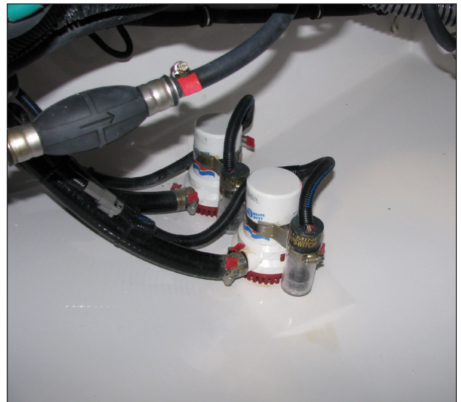
Aft Bilge Pumps & Automatic Switches
