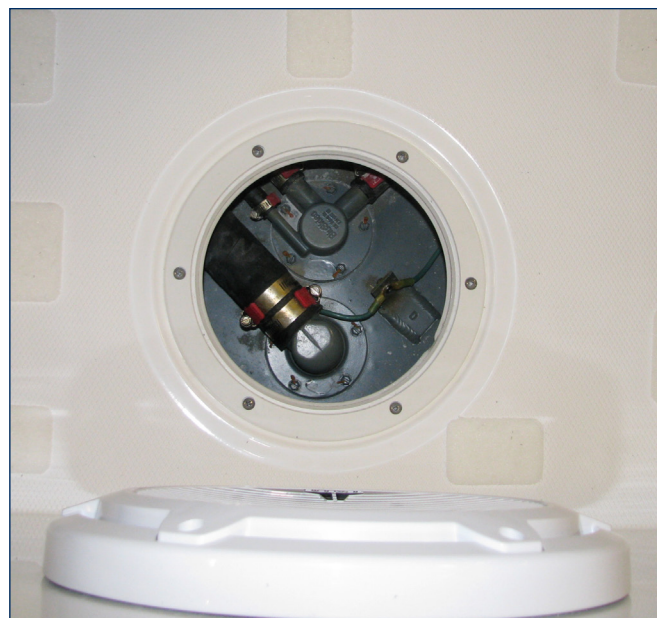
Fuel Fill & Vent Hose Connections
