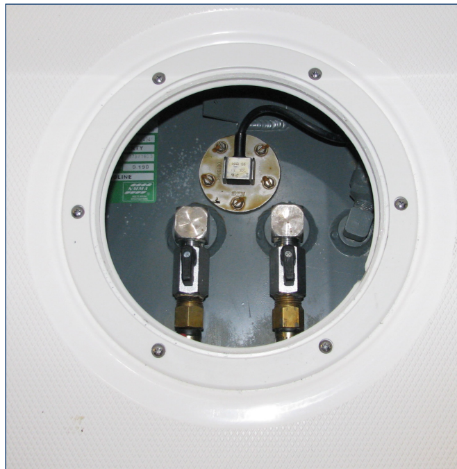
Fuel Withdrawal Valves & Tank Sending Unit
