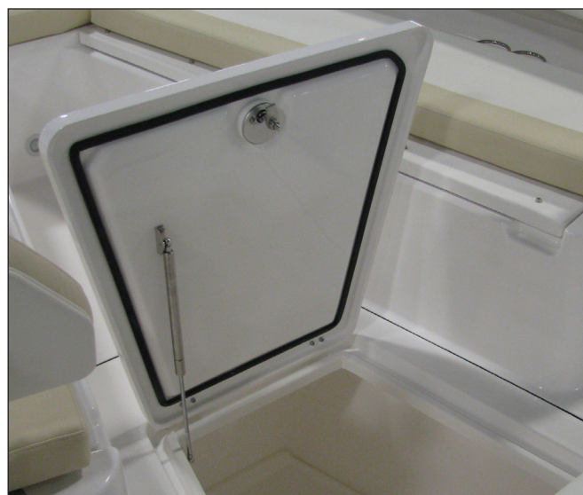
Hatch Twist Lock Latch & Gas Charged Spring
