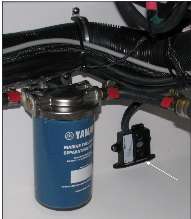
Bilge High Water Alarm Automatic Switch
