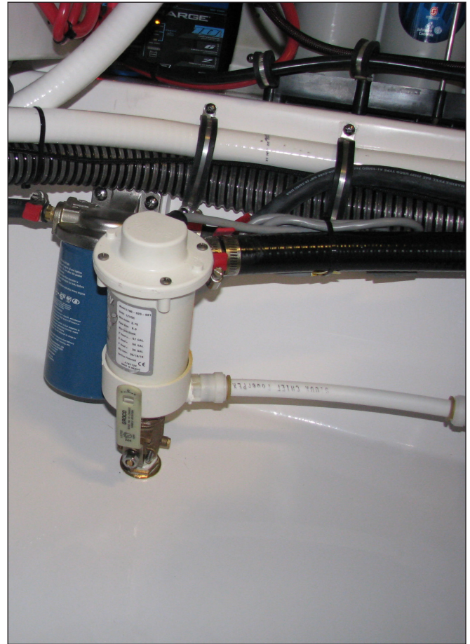
Baitwell Supply Pump & Seacock
