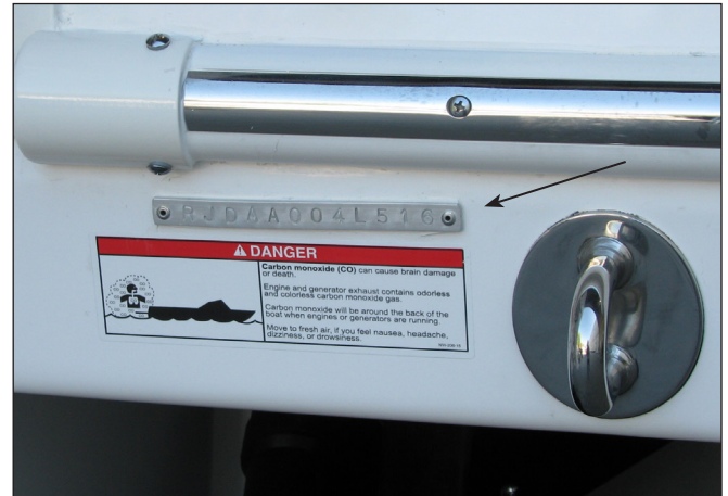
Hull ID # On Starboard Side of Transom
