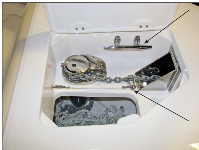
Windlass Chain Binder & Anchor Line Cleat
