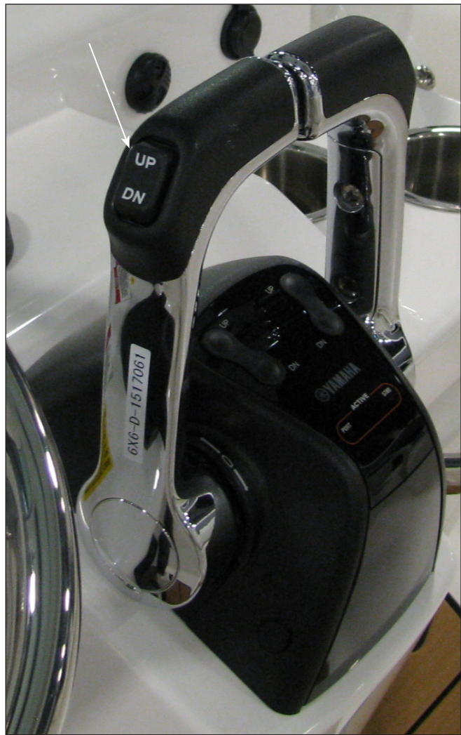
Twin Engine Control Engine Tilt & Trim Switch
