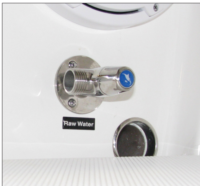
Typical Washdown Hose Connection
