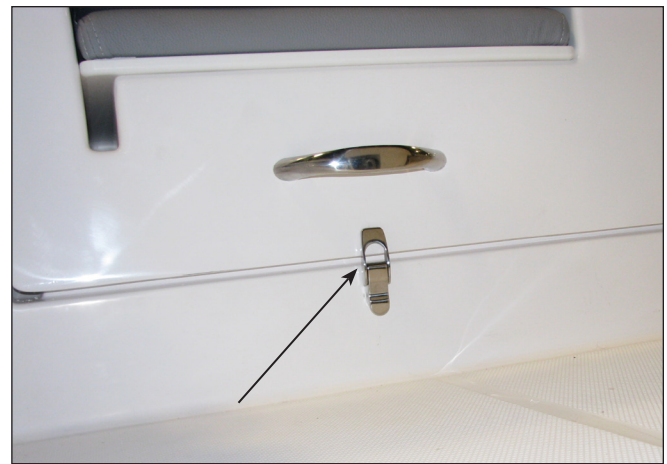
Stern Seat Base Cam Action Compression Latch
