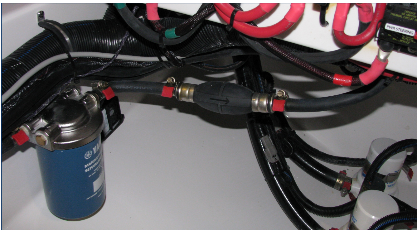
Typical Yamaha Fuel Filter & Primer Bulb
