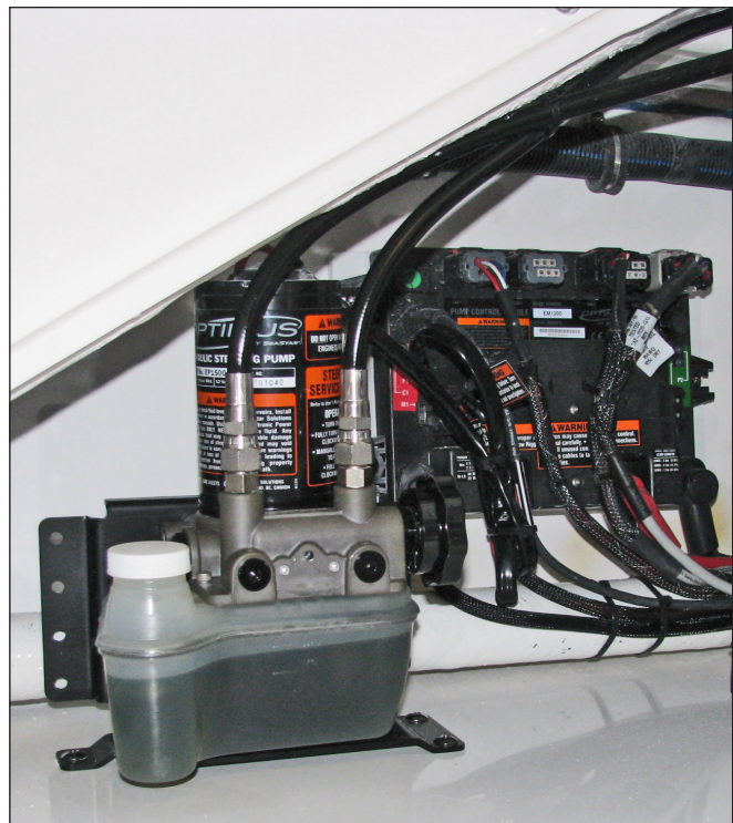
Typical Electronic Steering Unit
