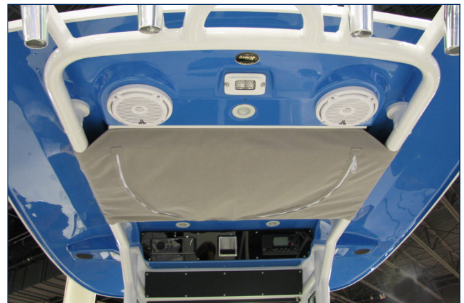
Hardtop Liner, Overhead Storage & Electronics Panel
