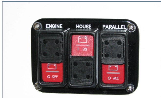
Remote Battery Switches
