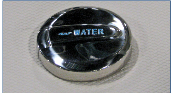
Fresh Water Fill
