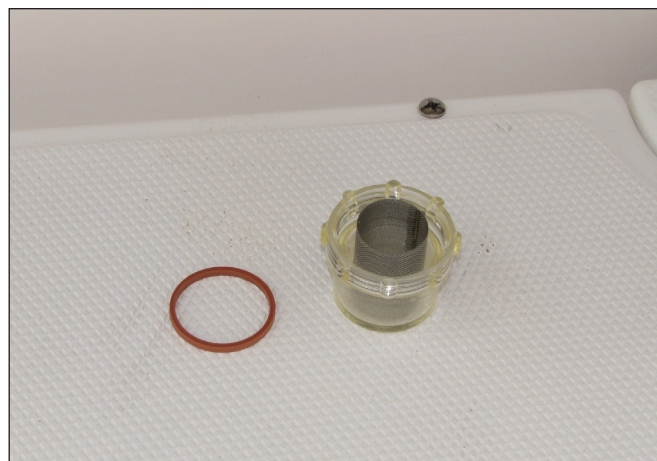
Typical Raw Water Pump Strainer Removed for Cleaning
