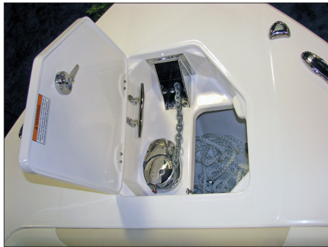
Windlass & Rope Locker
