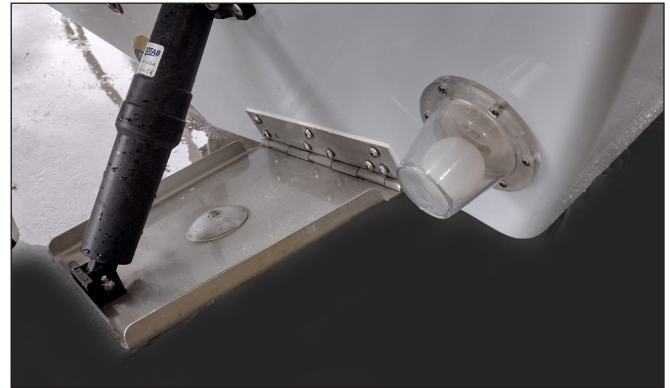
Scupper Drain Check Valve Assembly
