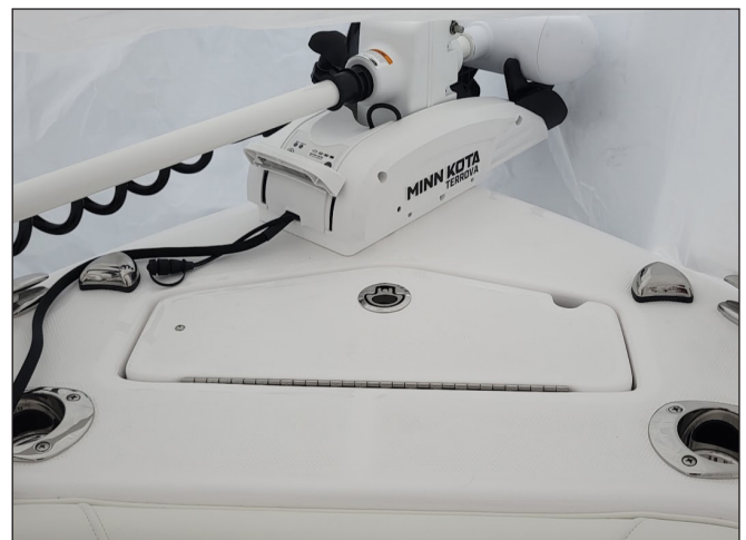
Anchor Rope Locker and Latch
