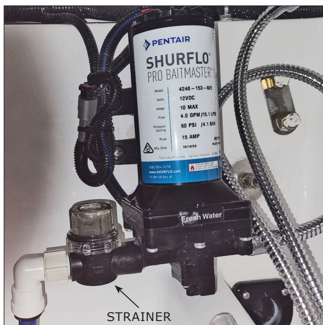
Typical Fresh Water Pump and Strainer
