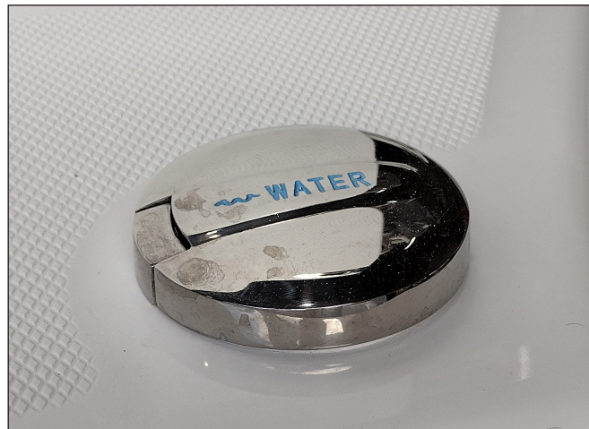
Fresh Water Fill
