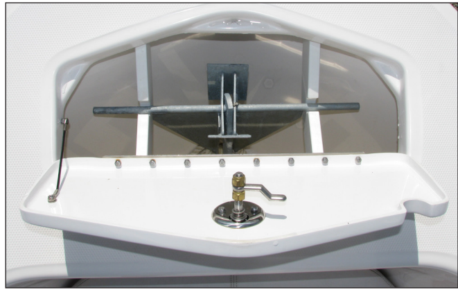
Anchor Properly Secured in Locker
