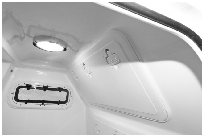
12 Volt Light, Port Window & Upper Rear Bulkhead Access Hatch
