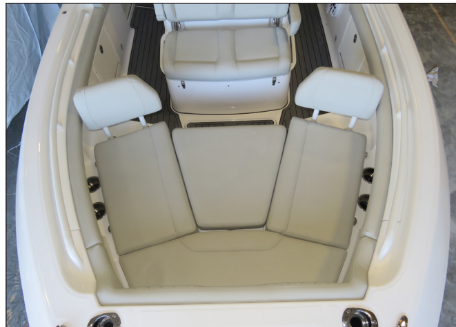
Casting Deck Converted to a Sun Lounge
