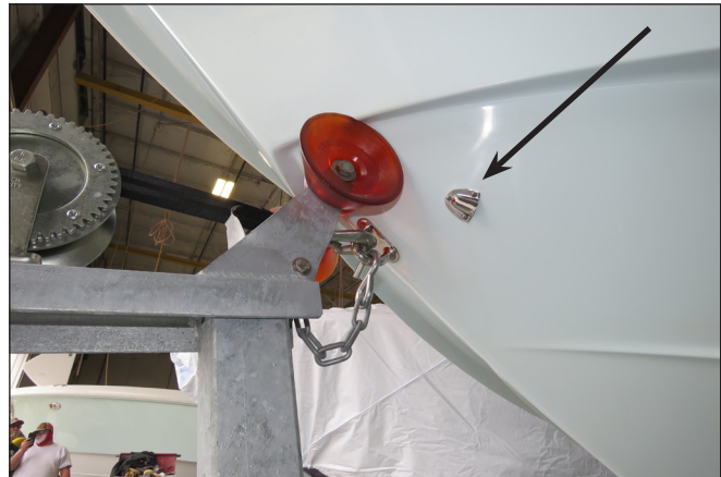
Rope Locker Drain
