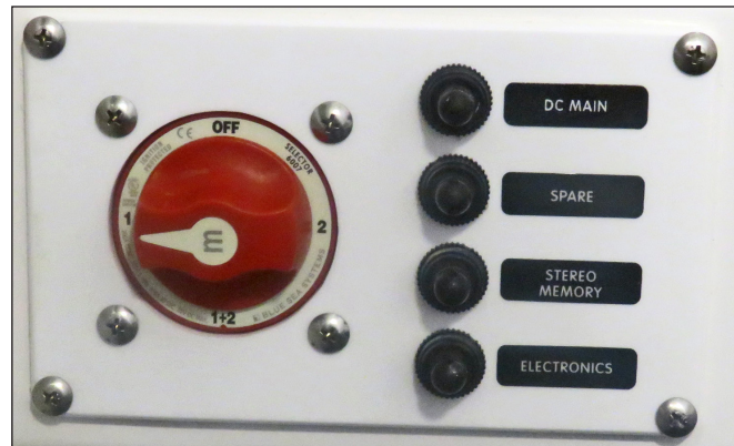
Battery Switch Panel Circuit Breakers
