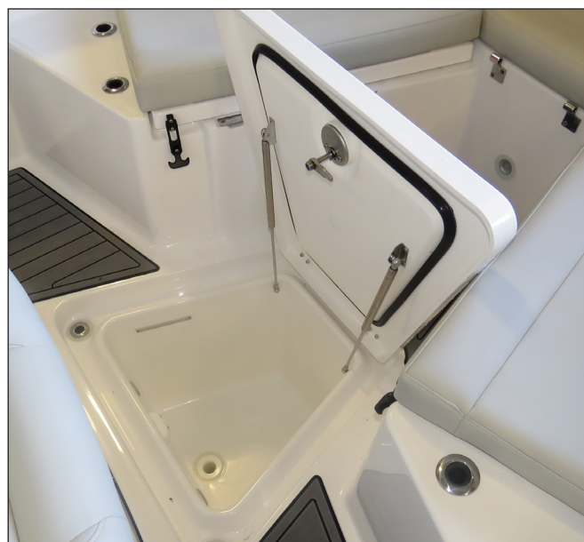
Hatch Twist Lock Latch & Gas Charged Spring
