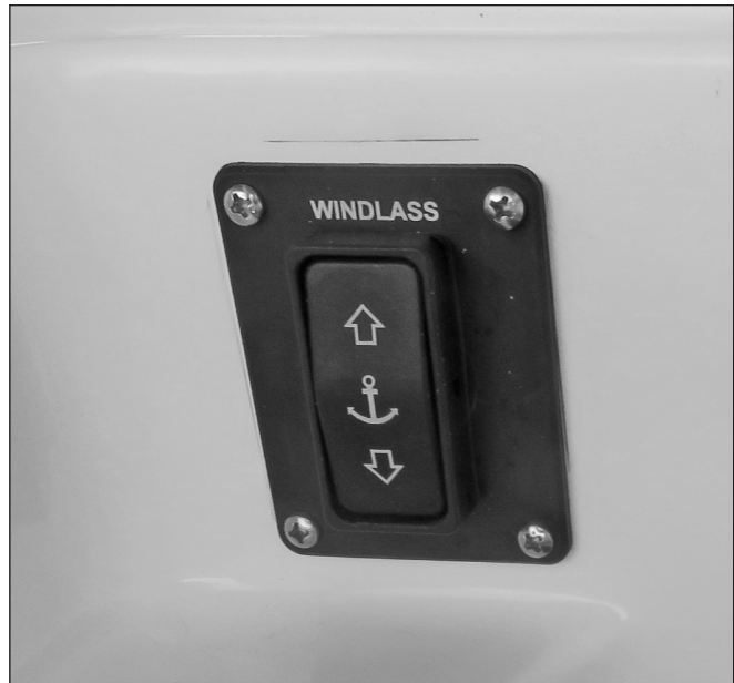
Windlass Rocker Switch in Windlass Compartment
