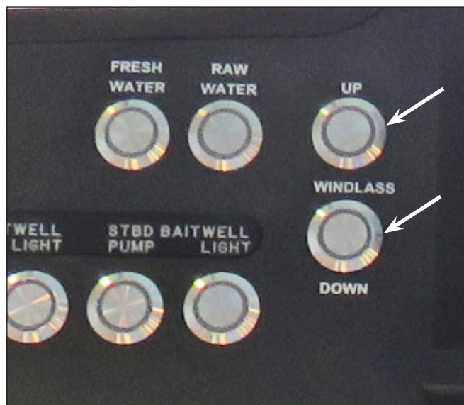
Windlass UP/DOWN Switches in Helm Switch Panel
