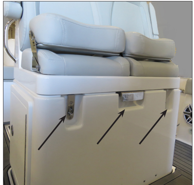
Helm Seat Pivot Latch and Sliding Bolt Latches
