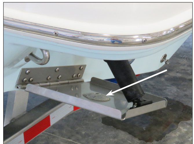
Zinc Anode Installed on Trim Tab Plane
