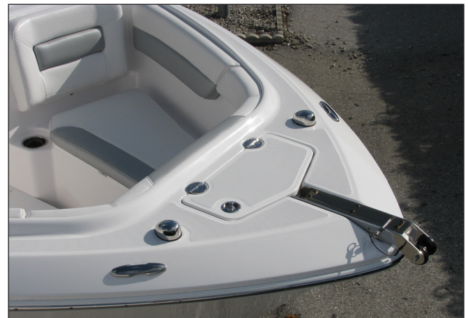
Anchor/Rope Locker and Roller Assembly
