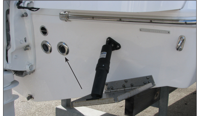
Transom Scupper Drain with Check Valve
