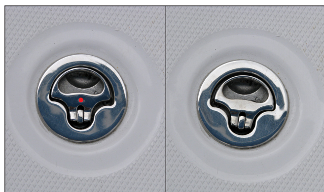
Hatch not Latched Red Dot Showing
