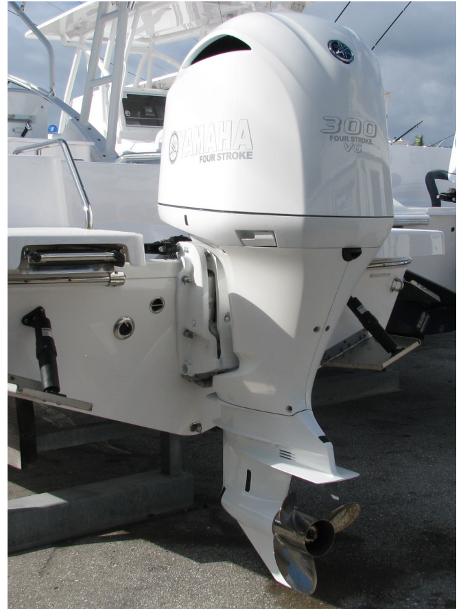
Outboard Power System
