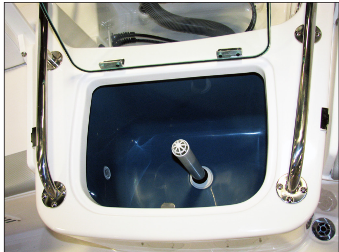
Baitwell and Overflow Pipe
