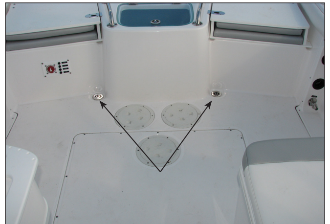
Cockpit Scupper Drains
