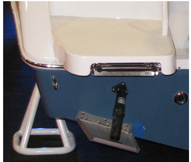
Typical Trim Tab Plane and Actuator
