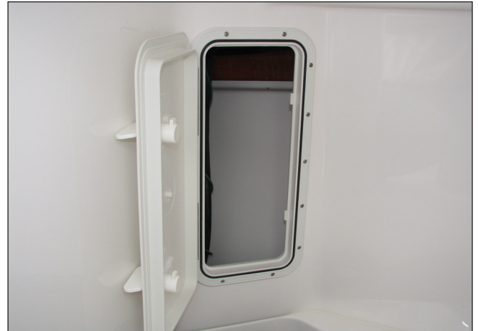
Bilge and Deck Component Access Panel
