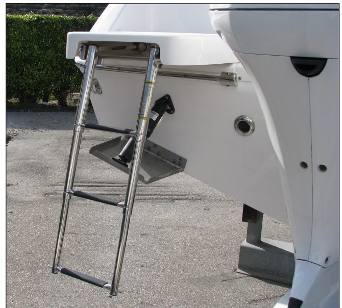
Boarding ladder Extended
