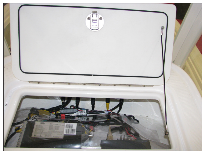
Top Step/Platform Open to Service Electronics
