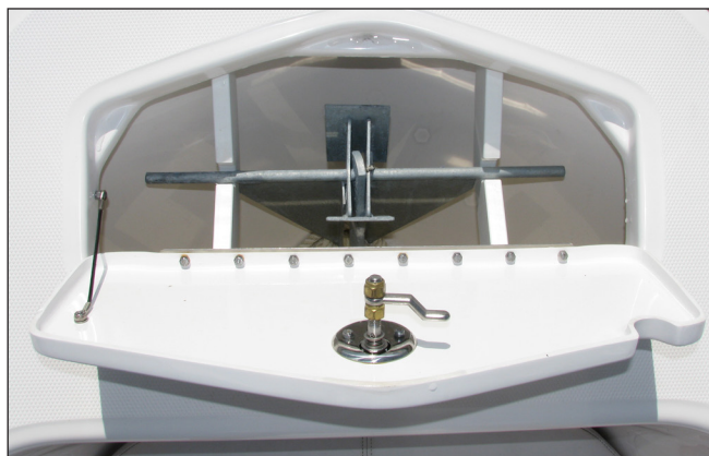
Anchor Properly Secured in Locker
