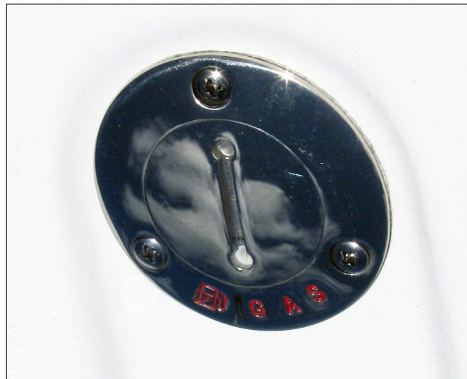
Typical Fuel Fill
