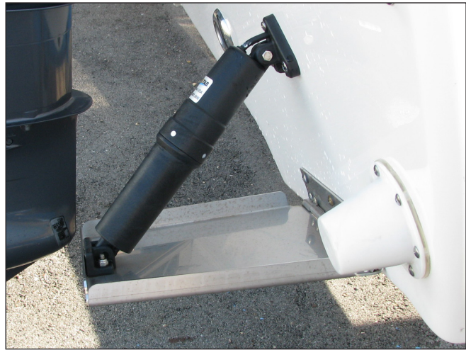
Typical Trim Tab Plane and Actuator
