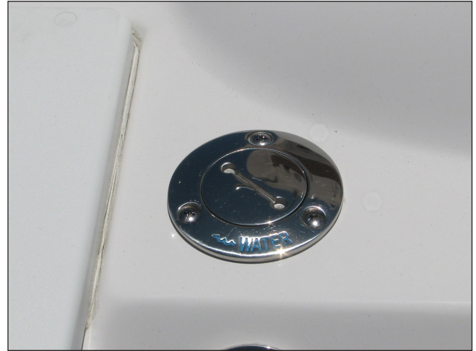
Fresh Water Fill
