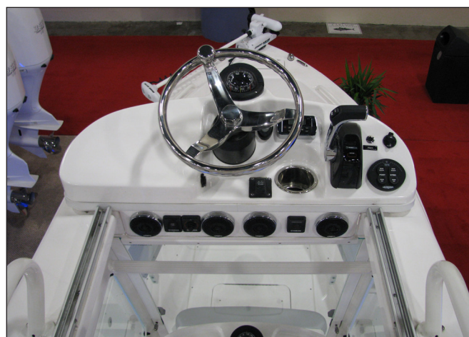
Upper Helm Station with Access Hatch/Seat Open
