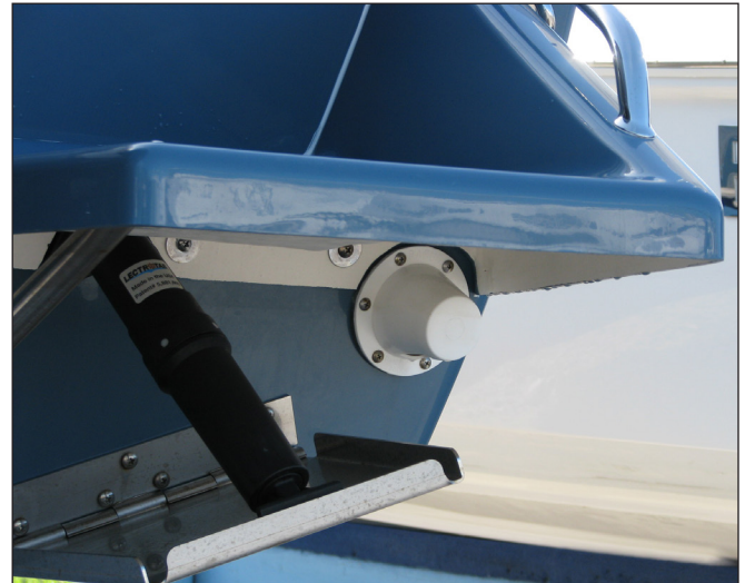
Scupper Drain Check Valve Assembly
