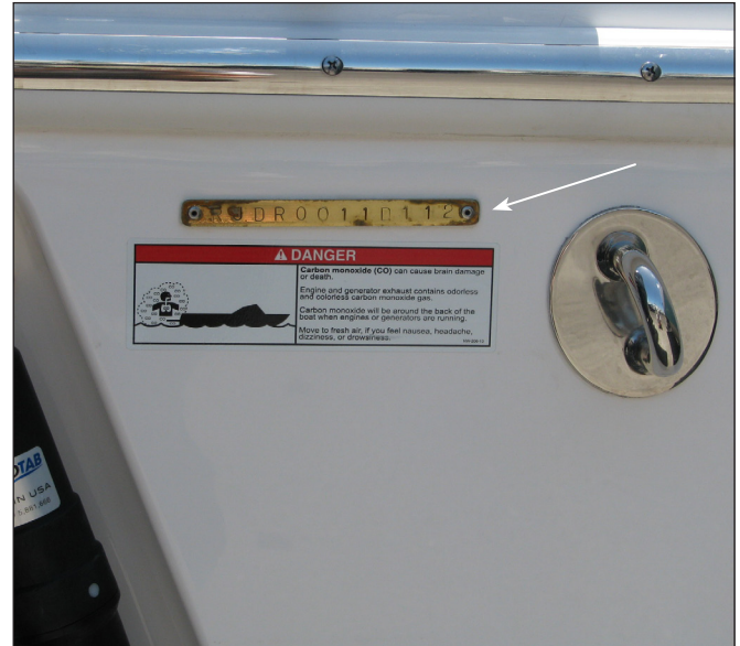
Hull ID # On Starboard Side of Transom
