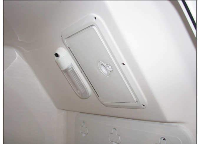
Upper Helm Access Hatch and Light Fixture
