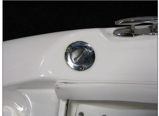
Fresh Water Fill
