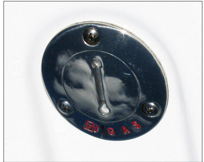
Typical Fuel Fill
