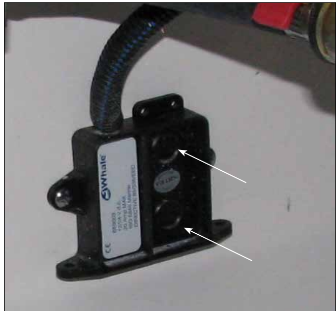
Bilge High Water Alarm Automatic Switch Recessed Test Discs
