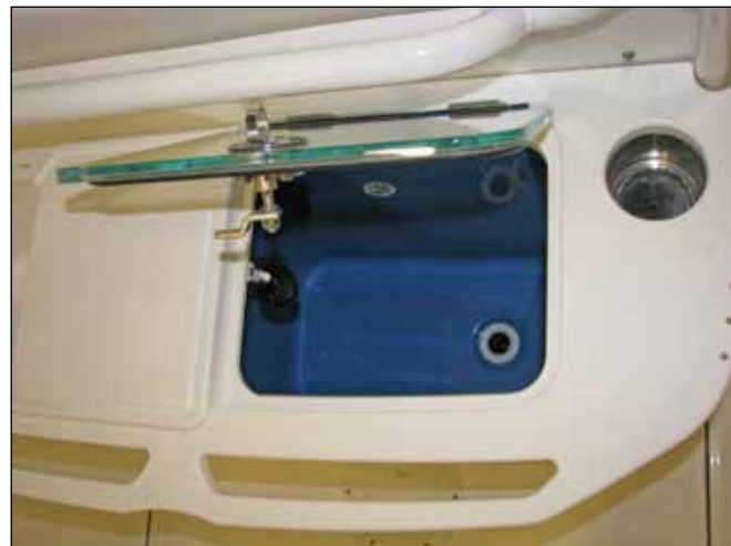
Baitwell Drain Fitting
