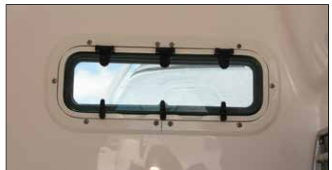
Cabin Port Window & Twist Action Locks
