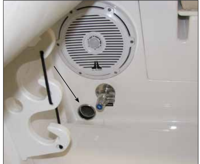
Cockpit Scupper Drain
