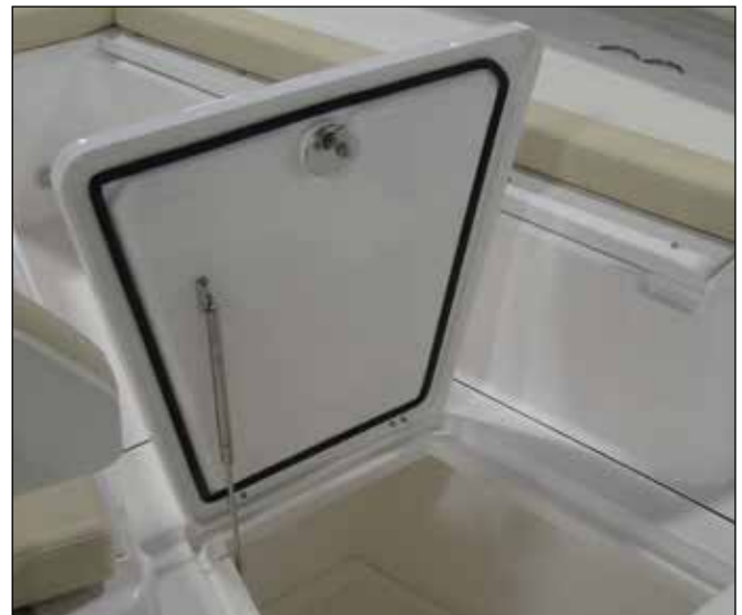
Hatch Twist Lock Latch & Gas Charged Spring
