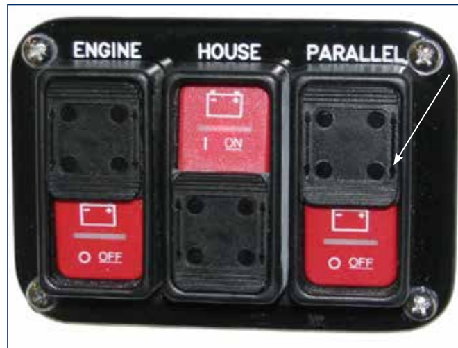
Single Engine Battery Parallel Switch
