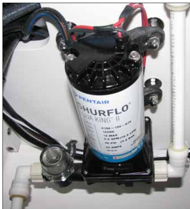
Raw Water Pressure Pump & Sea Strainer
