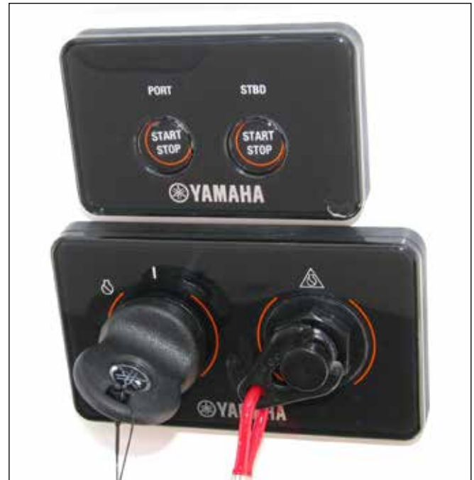
Typical Twin Engine Yamaha Command Link Ignition & Engine Start/Stop Switch System
