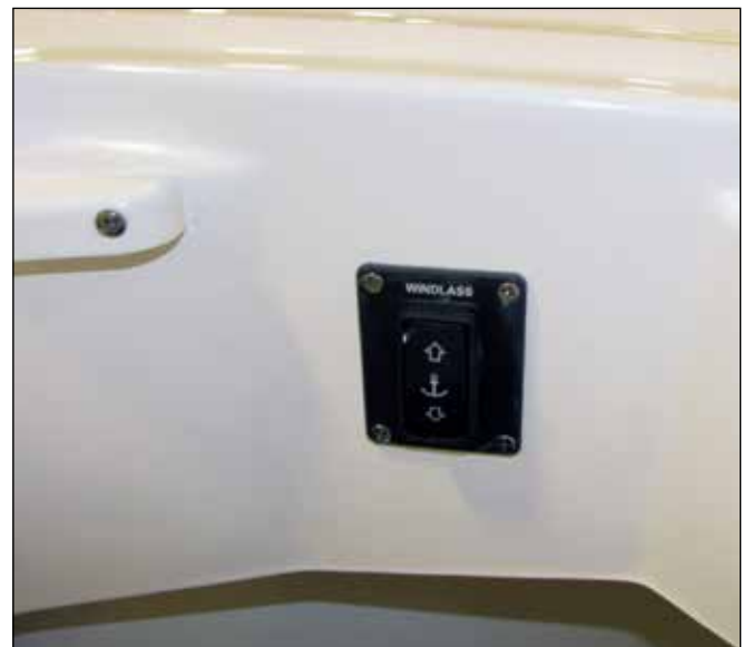
Anchor/Rope Locker Windlass Switch
