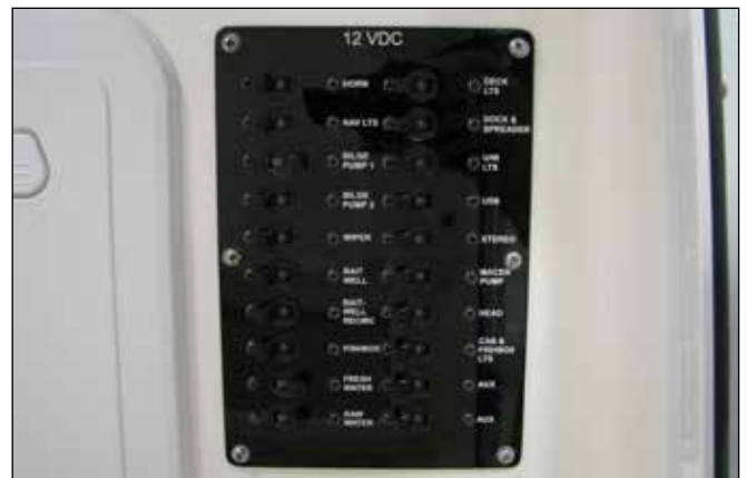
12 Volt Accessory Circuit Breakers
