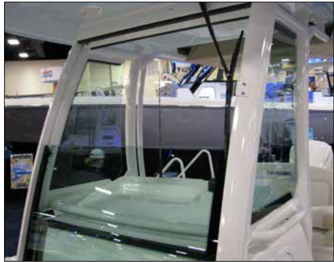
Opening Windshield in the Down Position
