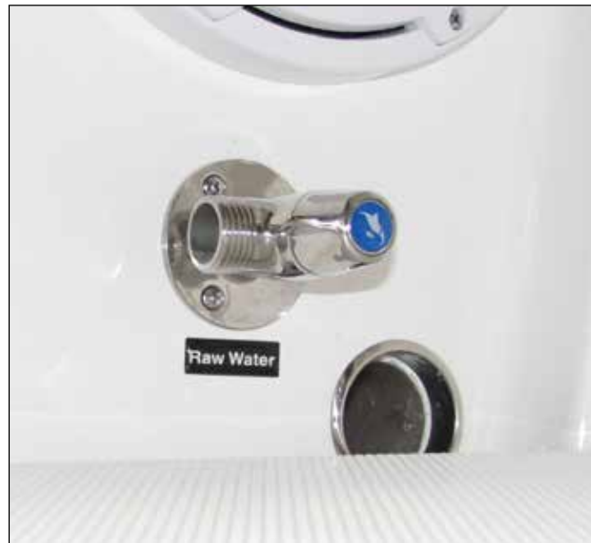
Typical Washdown Hose Connection
