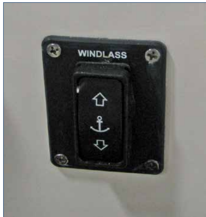
Anchor Locker Windlass Switch
