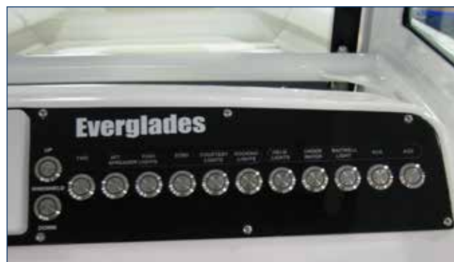
Starboard Side Helm Switches
