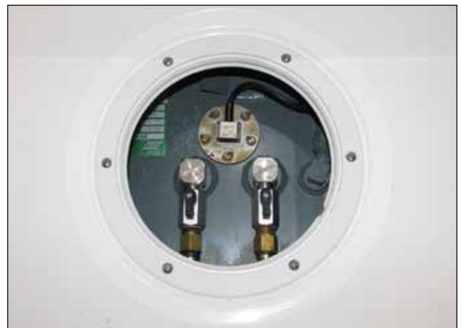
Typical Round Access Hatch In Cockpit
