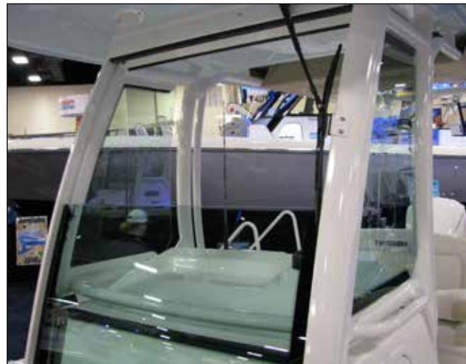
Opening Windshield In Open Position
