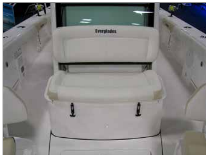
Forward Console Seat Draw Latches
