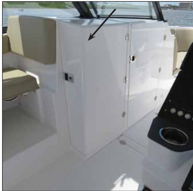
Port Console Cabin Door
