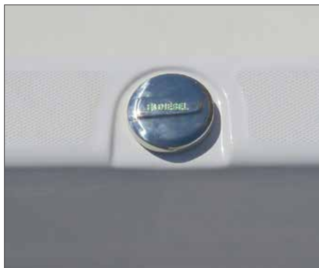
Diesel Fuel Fill
