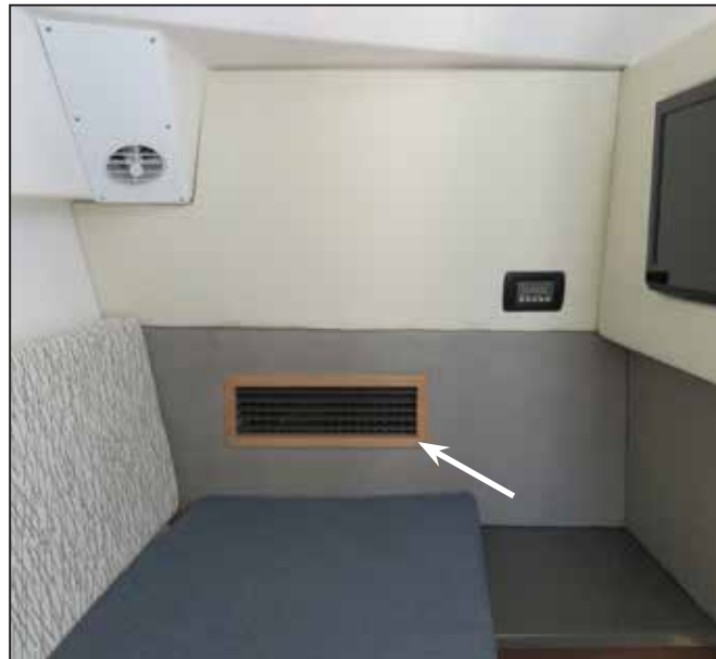
Air Condition Intake Vent
