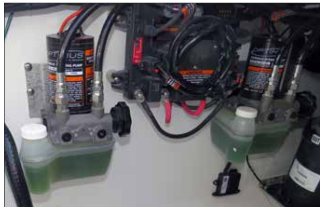
External Electronically Controlled Steering Pumps
