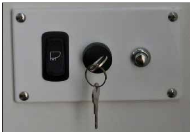
Waste Discharge Switch & Marine Toilet Control Switch in Head System Control Panel
