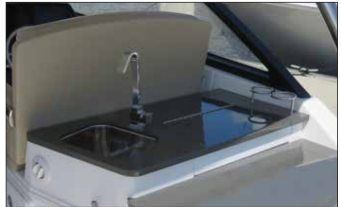
Galley Fresh Water Sink
