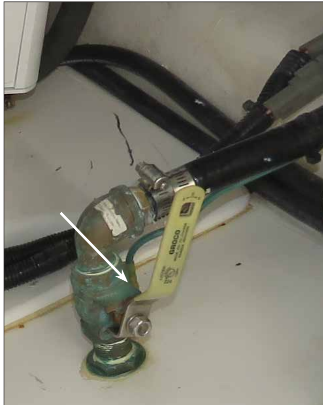
Typical Seacock Bonding Wire & Connection
