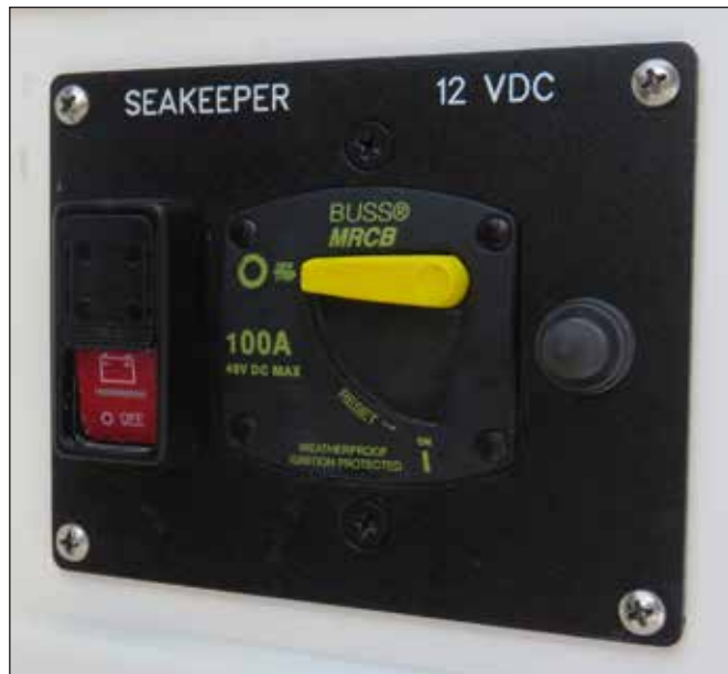
Seakeeper Battery Switch & Circuit Breaker Panel
