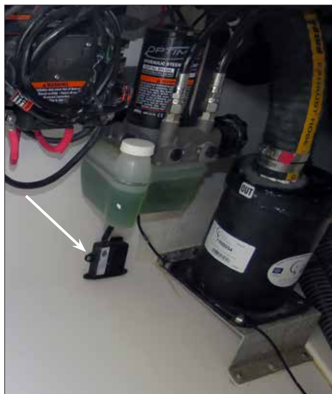
Bilge High Water Alarm Automatic Switch
