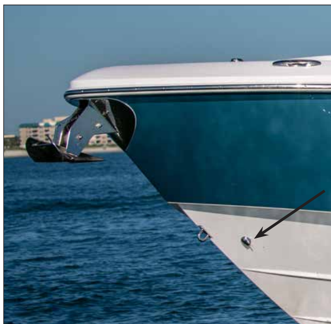
Rope Locker Drain Fitting in Hull Side
