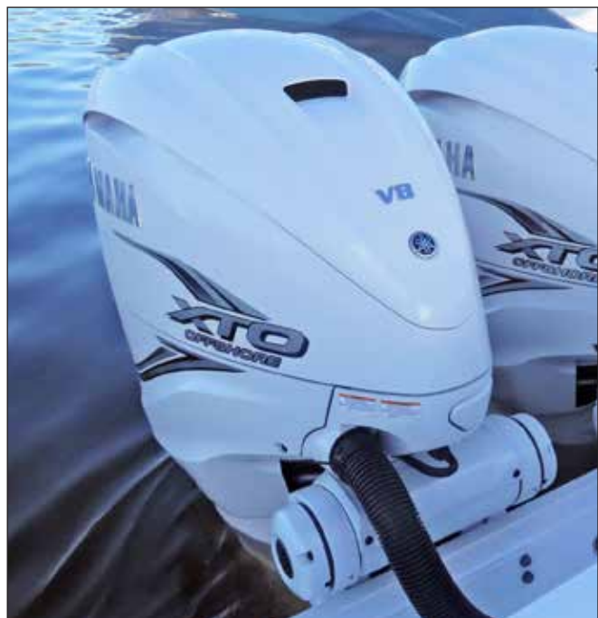
Helm Master Engine Mounted Electron Steering
