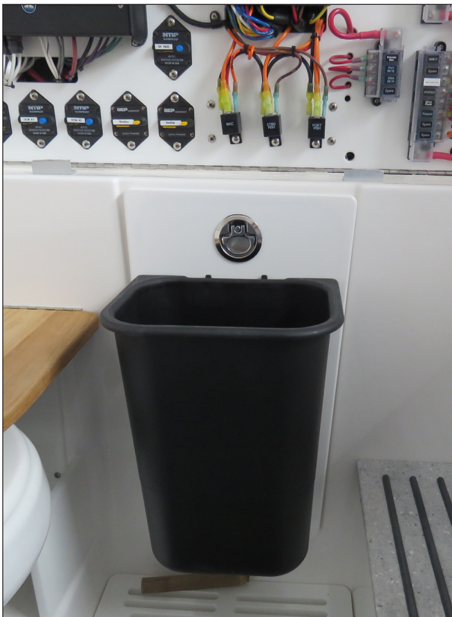
Head Compartment Basket & Removable Panel That Provides Access To Windshield Hydraulic Pump
