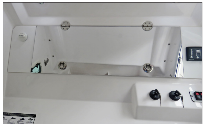
Upper Helm Equipment Access Door in Head Compartment
