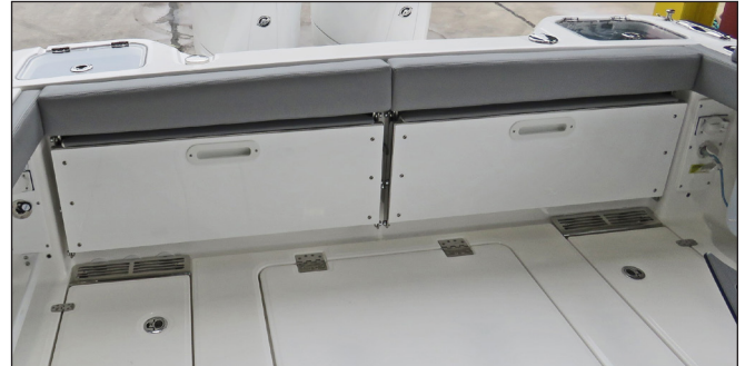
Typical Scupper Drains & Drain Rails
