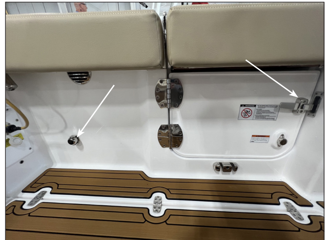
Side Boarding Door and Gate Closed Magnetic Latch & Door Latch w/ Safety Pin
