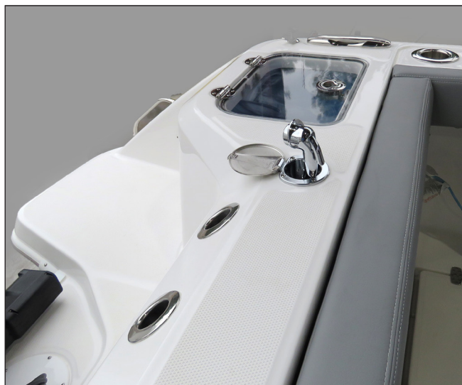
Aft Cockpit Fresh Water Shower
