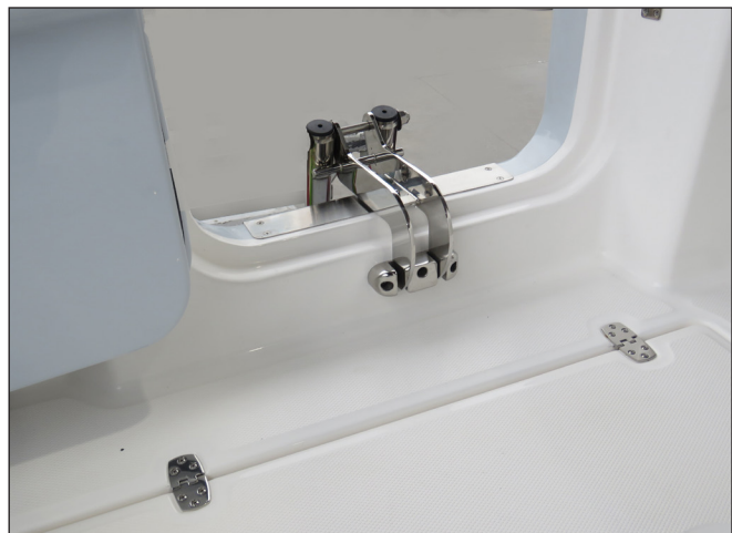
Ladder Secured To Side Door Bracket
