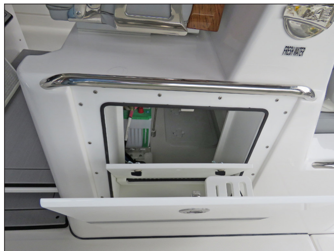
House Battery Compartment Access
