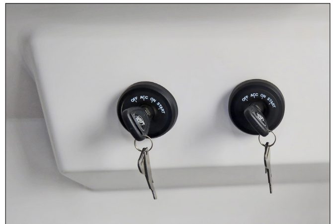
Typical Mercury Ignition Switches On Aft Head Compartment Bulkhead
