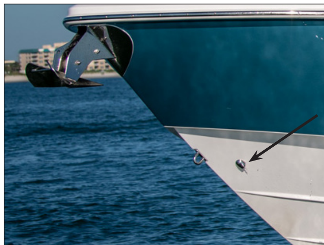
Rope Locker Drain Fitting in Hull Side
