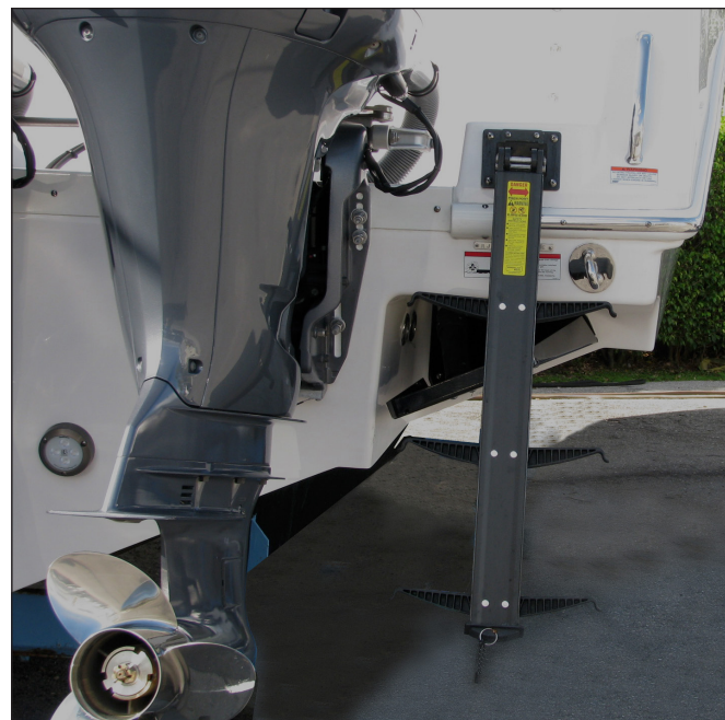
Typical Stern Ladder Deployed
