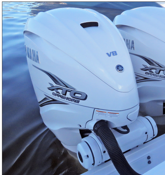
Helm Master Engine Mounted Electron Steering
