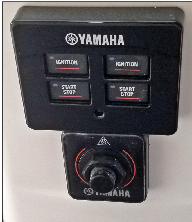
Yamaha Digital Ignition Emergency Stop Switch & Start/Stop Buttons
