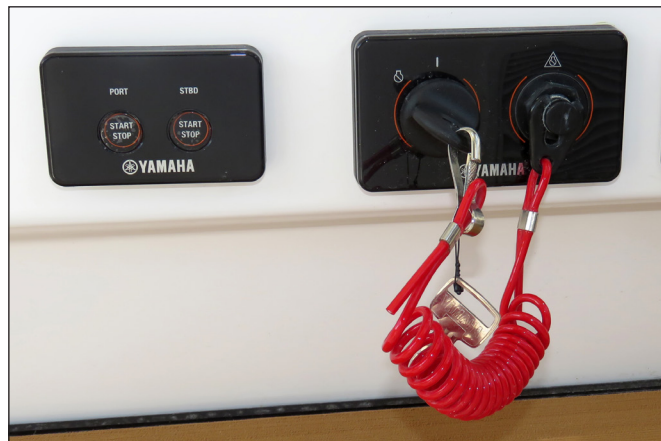
Yamaha Key Ignition Switch, Emergency Stop Switch, Lanyard & Start/Stop Buttons
