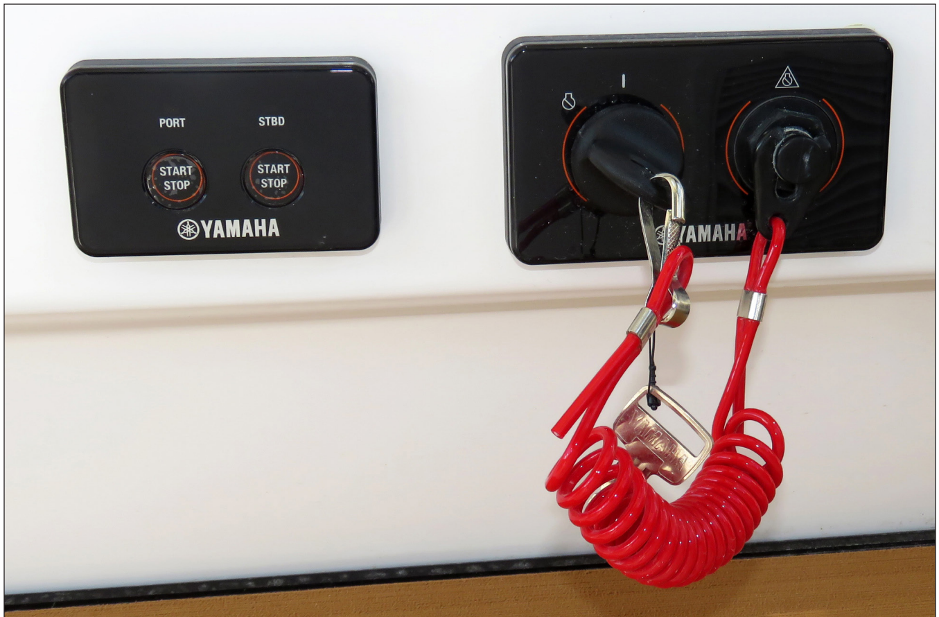
Typical Yamaha Twin Engine Ignition Switch & Start/Stop Buttons
