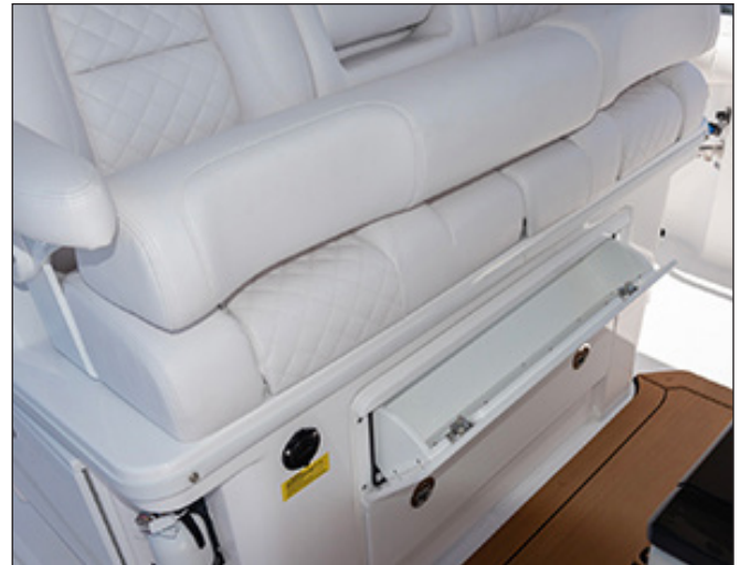
Helm Seat Bolsters Up Battery Switch & Circuit Breaker Access Doors Below Seats
