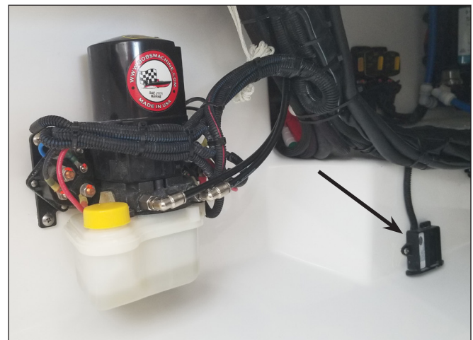
Bilge High Water Alarm Automatic Switch
