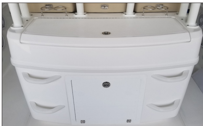
Electrical Systems Compartment Door
