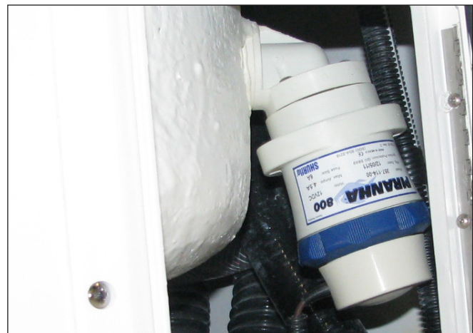
Typical Livewell Recirculation Pump
