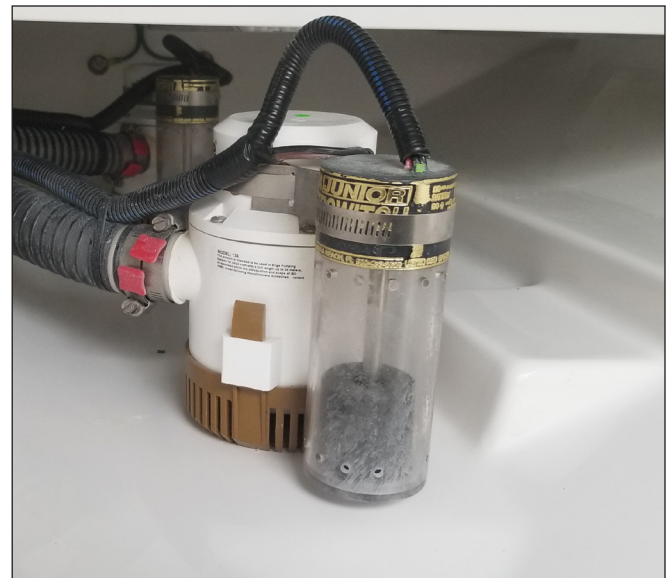
Aft Bilge Pumps & Automatic Switches
