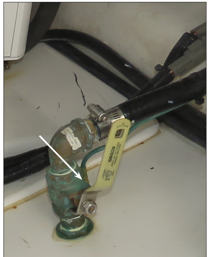
Typical Seacock Bonding Wire & Connection
