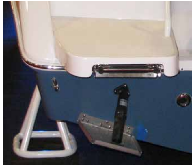
Typical Trim Tab Plane and Actuator
