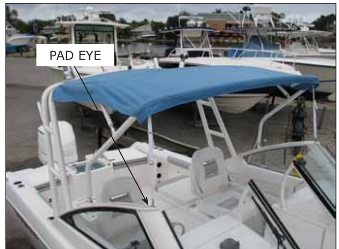
Arch Bimini Top Open with Forward Straps attached to Windshield Pad Eyes
