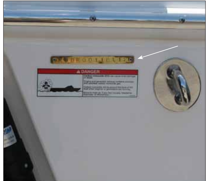
Hull ID # On Starboard Side of Transom
