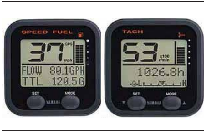
Typical Command Link® Tachometer and Speed Instruments
