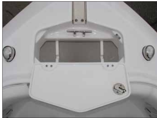
Anchor Cradle and Anchor Line Cleat
