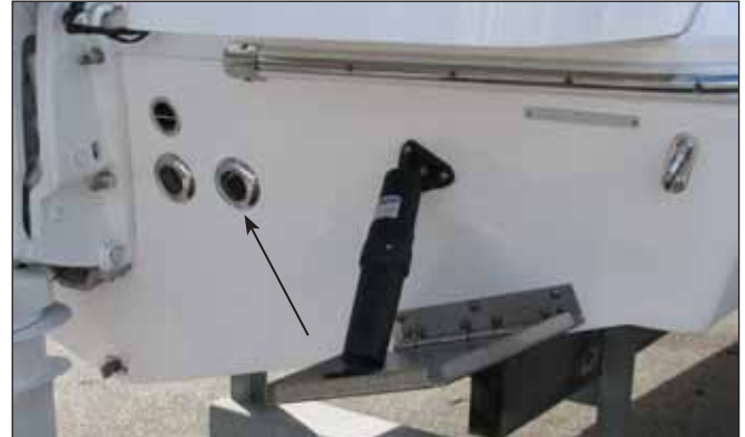
Transom Scupper Drain with Check Valve
