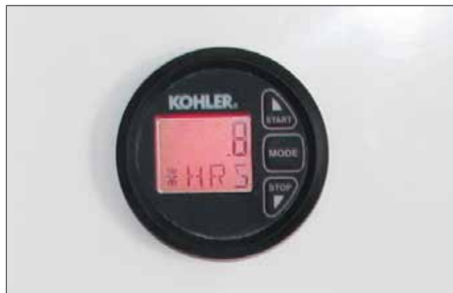
Cabin Generator Control Switch & Monitor
