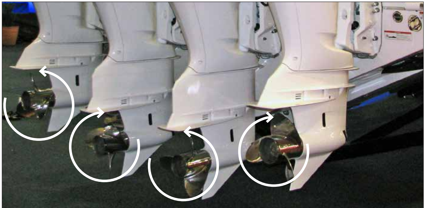
Typical Quad Engine & Propeller Rotation
