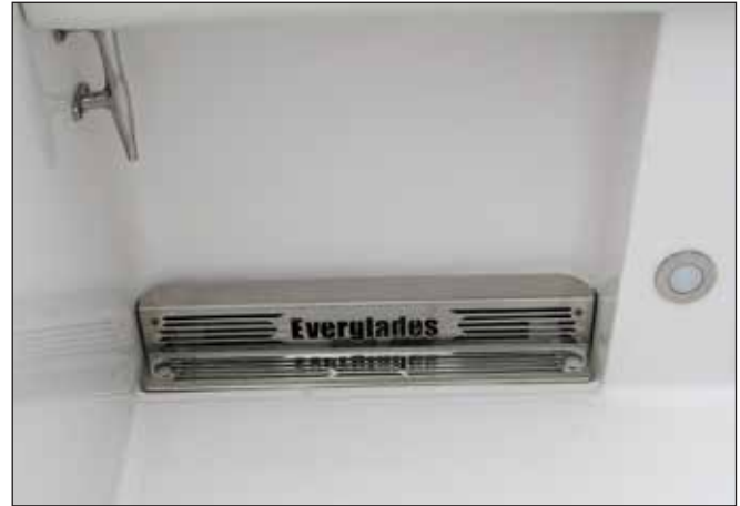
Typical Scupper Drains & Drain Rail
