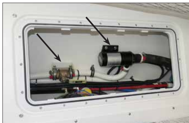
Overboard Macerator Pump & Thru-Hull Valve
