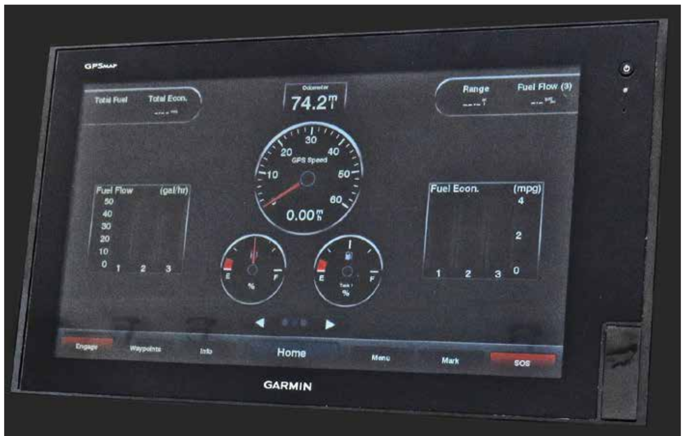
Typical Engine Gauge Display On A Garmin Chartplotter Screen
