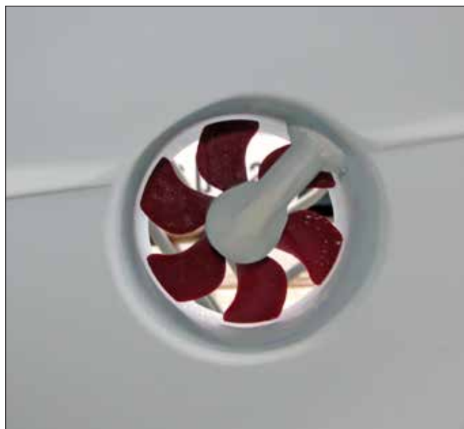
Typical Bow Thruster Drive Unit, propeller & tunnel
