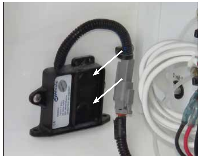
High Water Alarm Automatic Switch & Test Recesses
