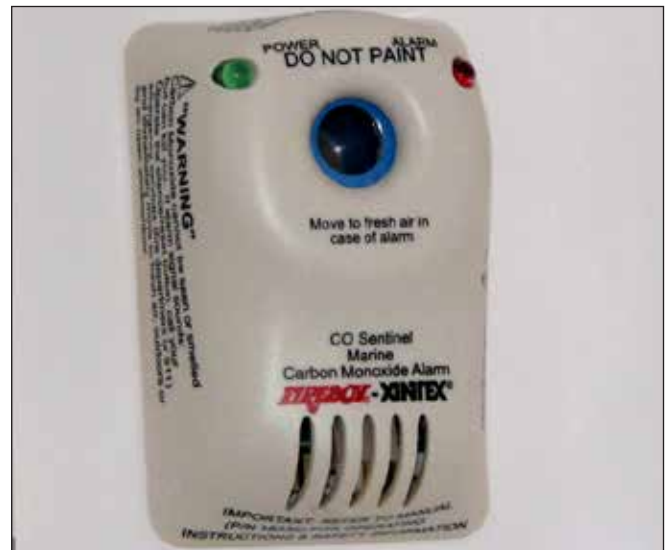
Typical Carbon Monoxide Detector & Alarm
