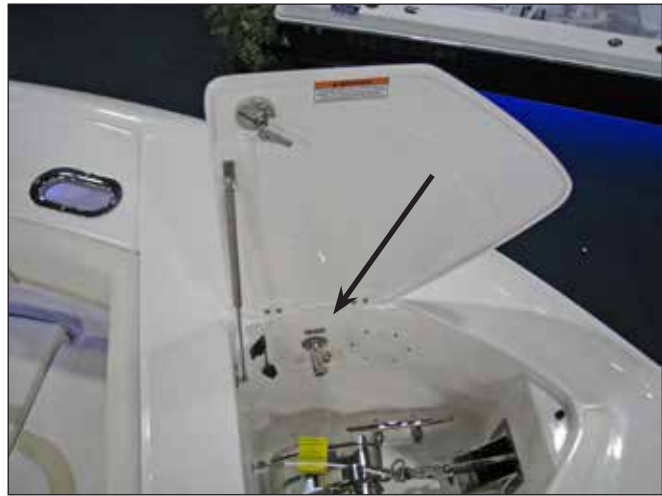
Windlass Raw Water Washdown Hose Connection
