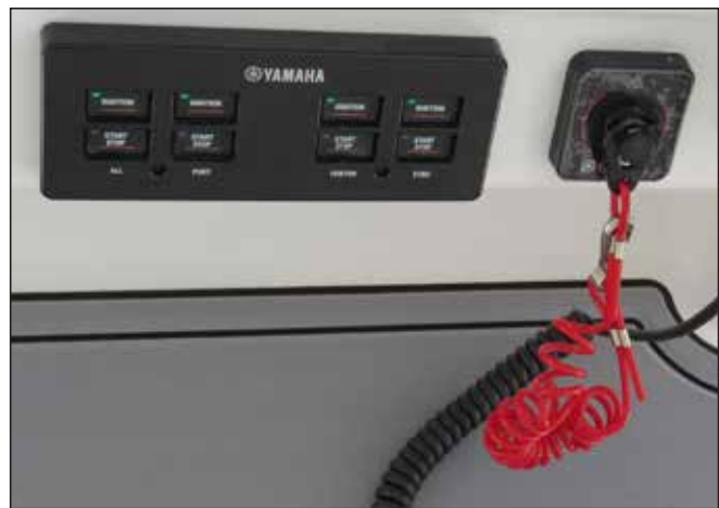
Yamaha Triple Engine Stop Switch & Lanyard Ignition START/STOP Switches
