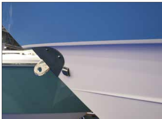
Rope Locker Drain Fitting in Hull Side
