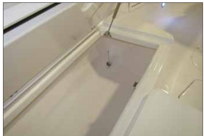
Bow Storage Compartment Drain & Drain Plug
