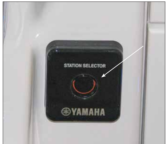
Typical Yamaha Triple Engine Station Transfer Button
