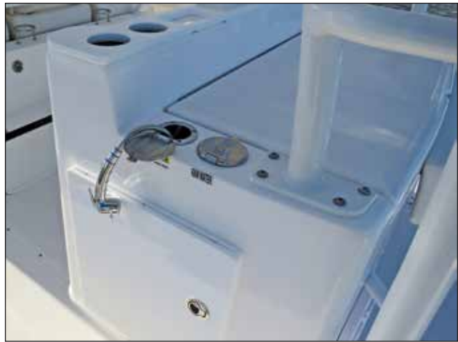
Cockpit Fresh Water Shower in Work Station
