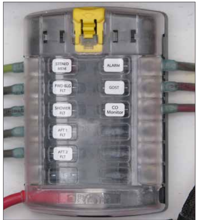
Continuous Power Fuse Panel
